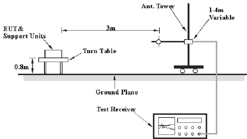
The radiated emission tests were performed in the 3-meter chamber test site, using the setup accordance with the ANSI C63.10-2020.
