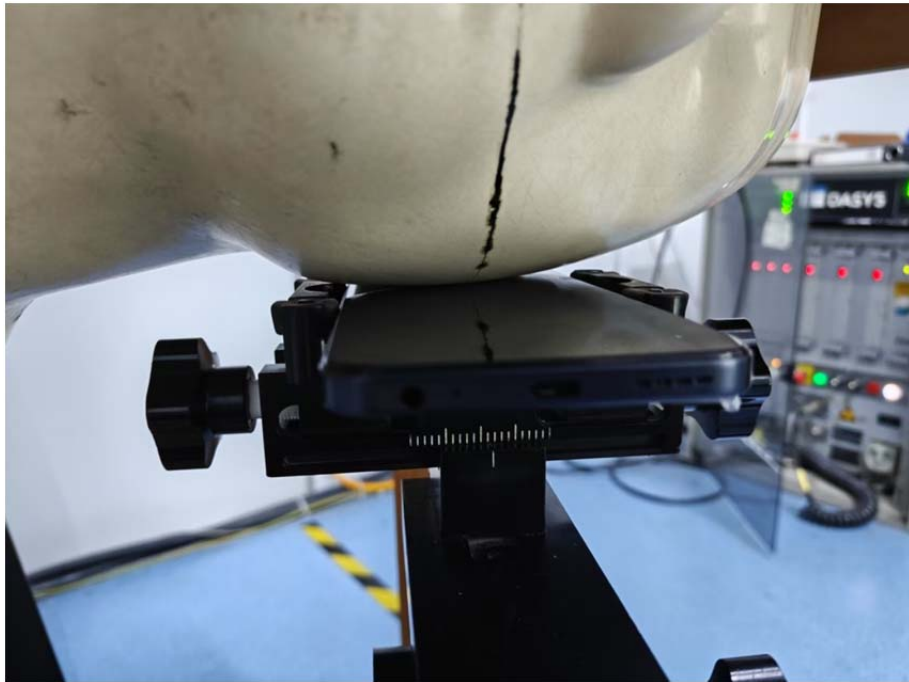
Head Left Tilt Setup Photo (0mm)
