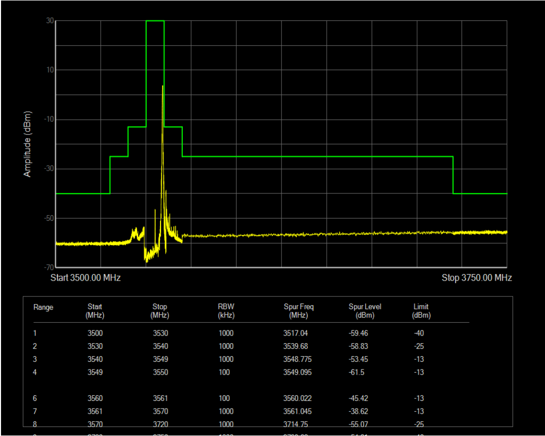
n77(3550-3700) SCS=30kHz CP_QPSK BW=10MHz Channel=637000 RB=24@0
