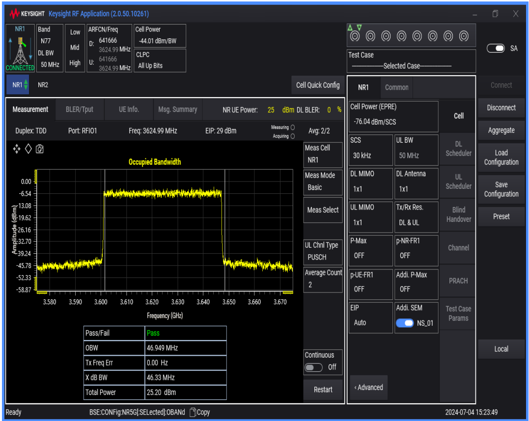
n77(3550-3700) SCS=30kHz DFT_QPSK BW=60MHz Channel=641666 RB=162@0
