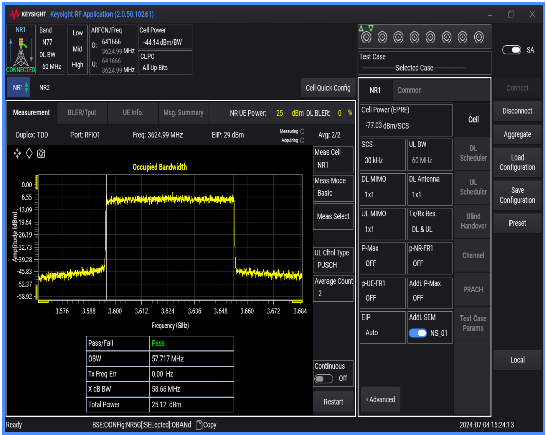
n77(3550-3700) SCS=30kHz DFT_QPSK BW=80MHz Channel=641666 RB=216@0
