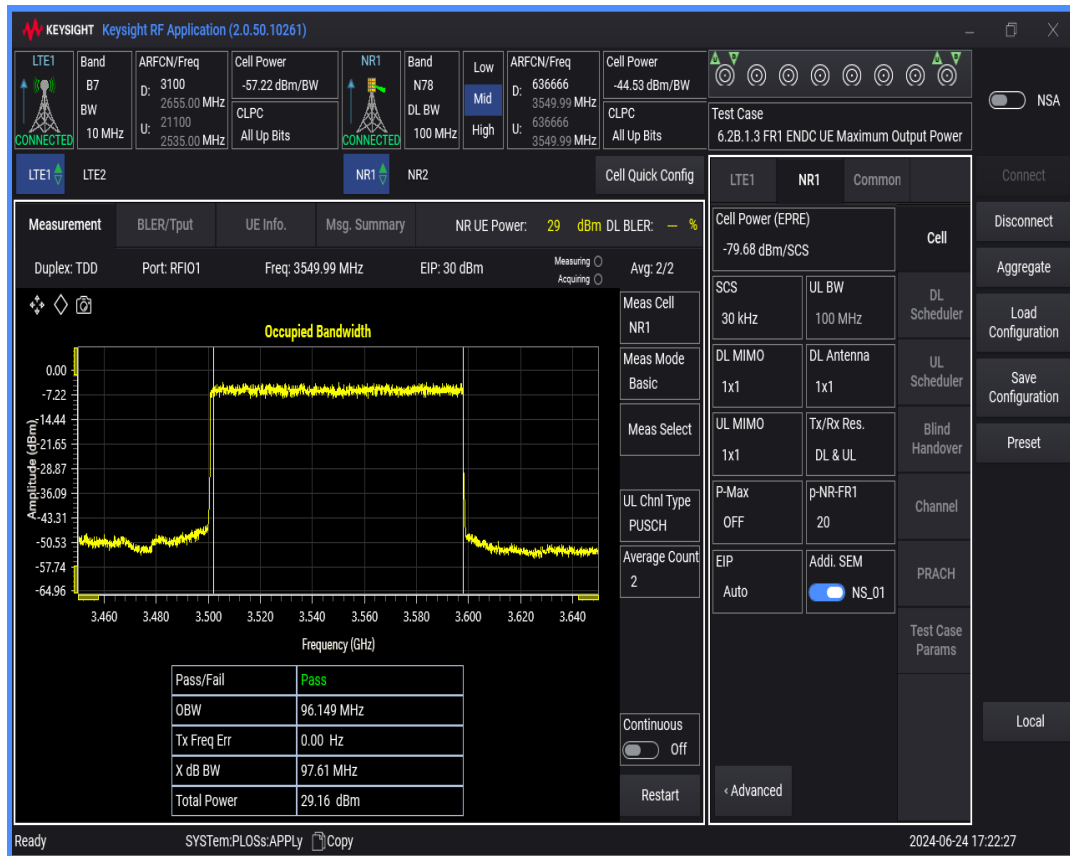
n78 SCS=30kHz DFT_BPSK BW=10MHz Channel=636666 RB=24@0
