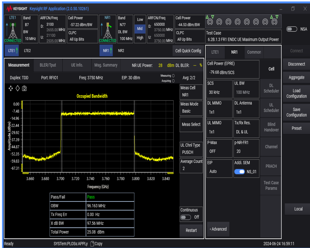
n77 SCS=30kHz DFT_BPSK BW=10MHz Channel=650000 RB=24@0
