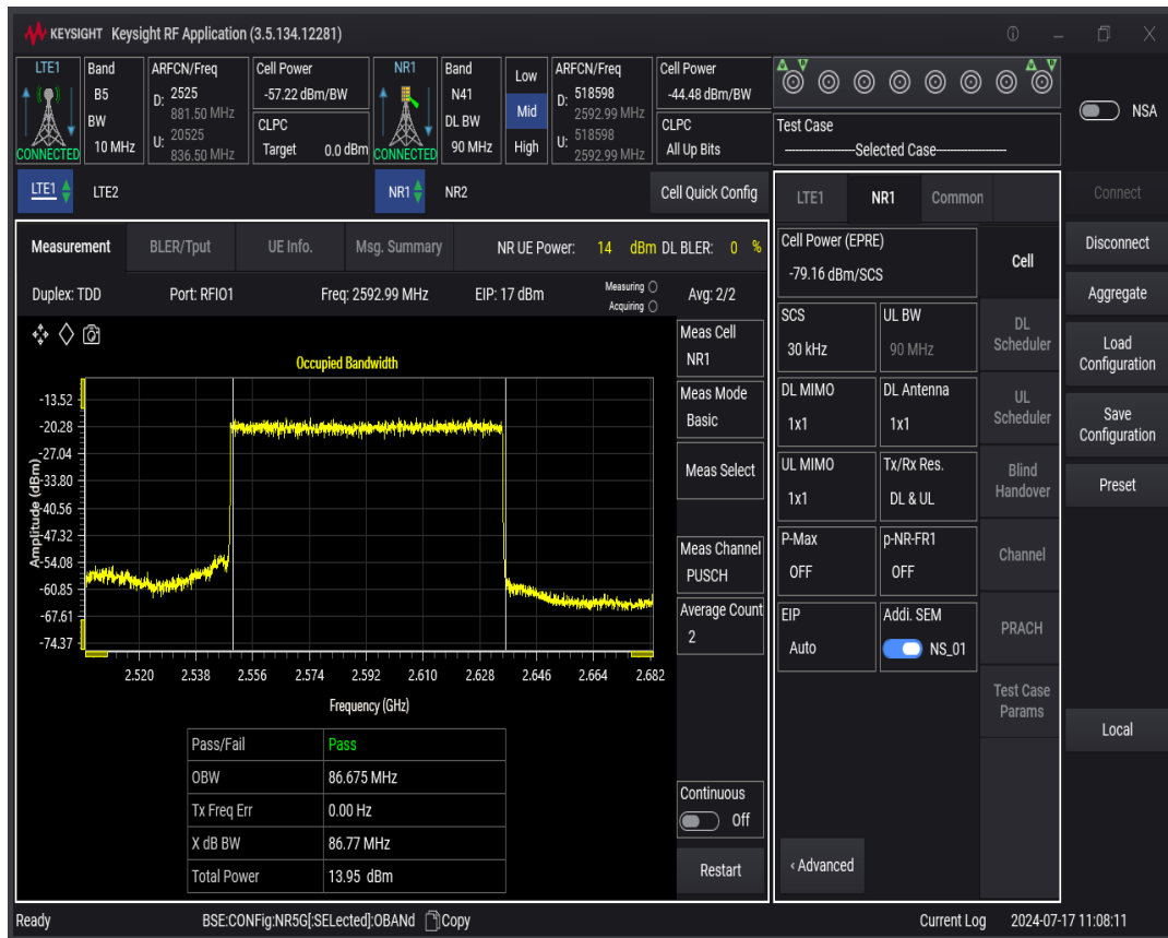
n41 SCS=30kHz DFT_QAM16 BW=100MHz Channel=518598 RB=270@0
