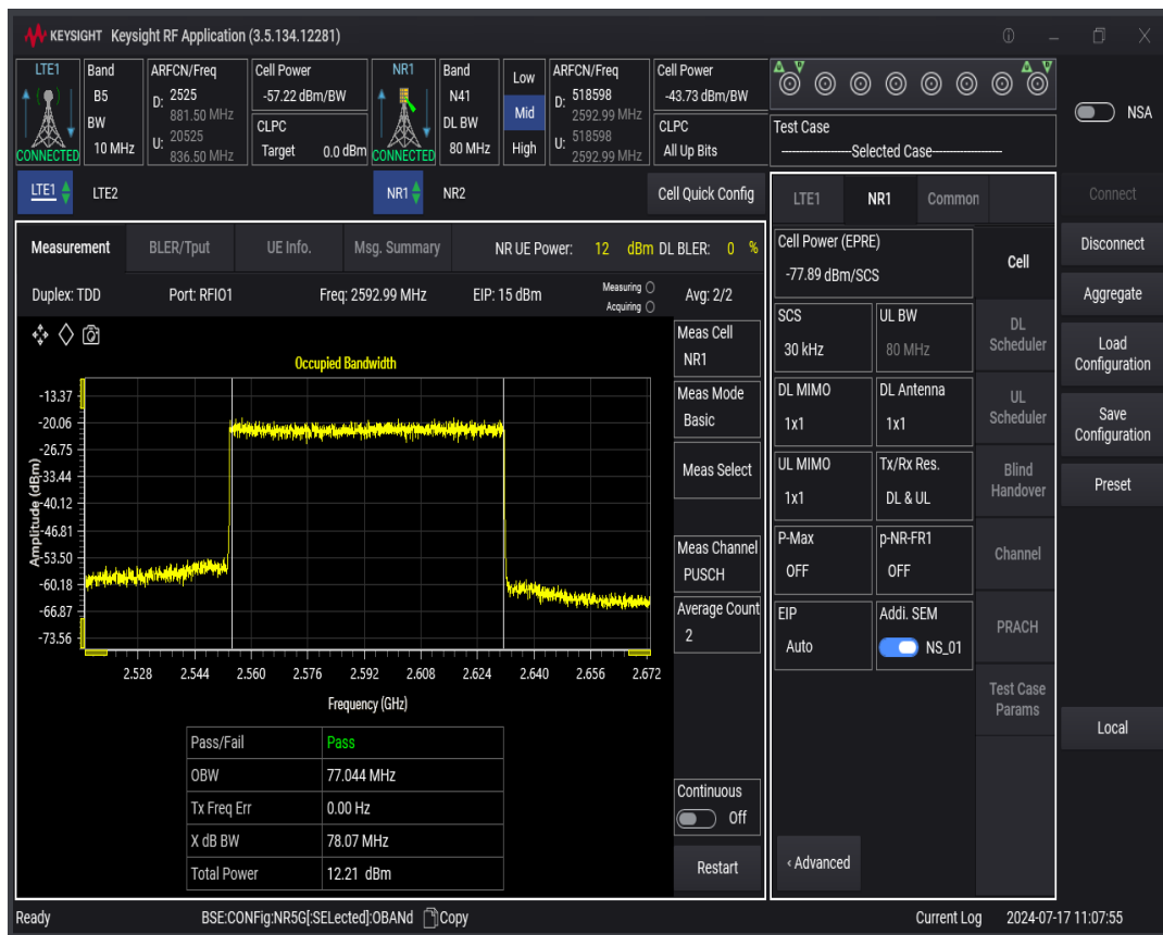
n41 SCS=30kHz DFT_QAM64 BW=90MHz Channel=518598 RB=240@0
