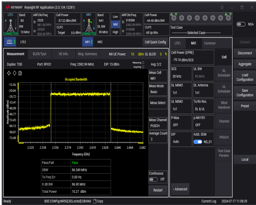
n41 SCS=30kHz DFT_QAM64 BW=100MHz Channel=518598 RB=270@0
