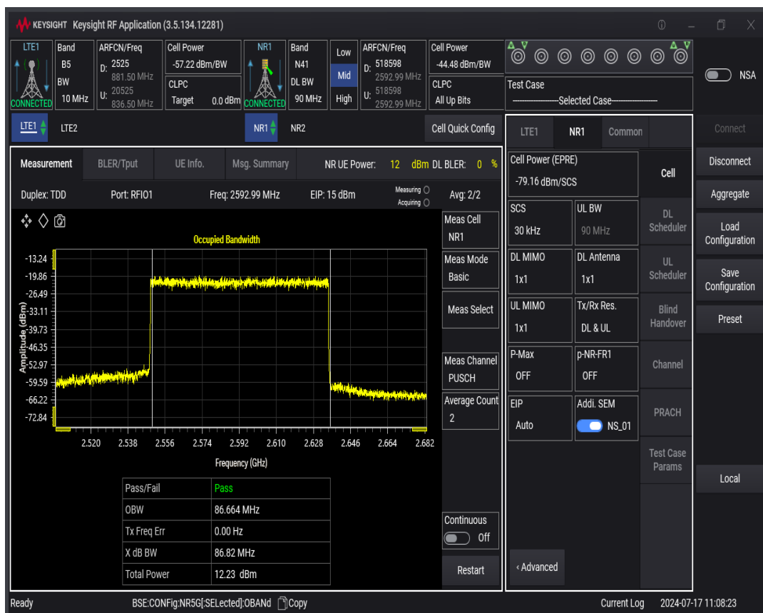
n41 SCS=30kHz DFT_QPSK BW=100MHz Channel=518598 RB=270@0
