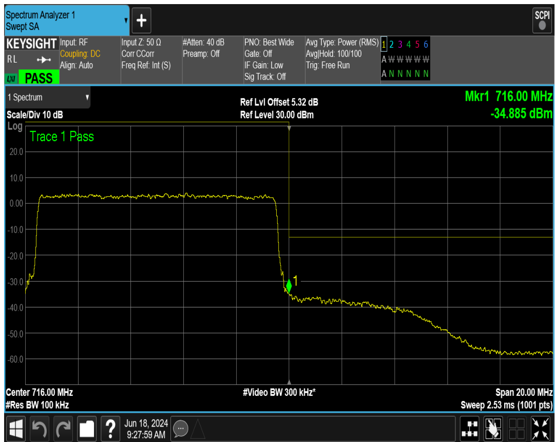
Band17 QPSK BW=5MHz Channel=23755 RB Size=25 Position=#0
