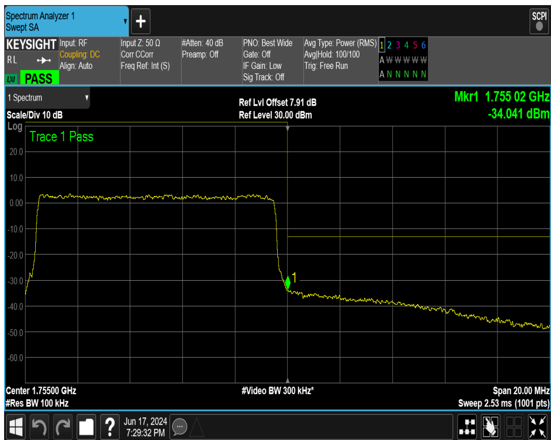
Band4 QAM16 BW=15MHz Channel=20025 RB Size=75 Position=#0
