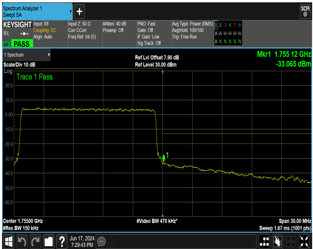
Band4 QPSK BW=20MHz Channel=20050 RB Size=100 Position=#0
