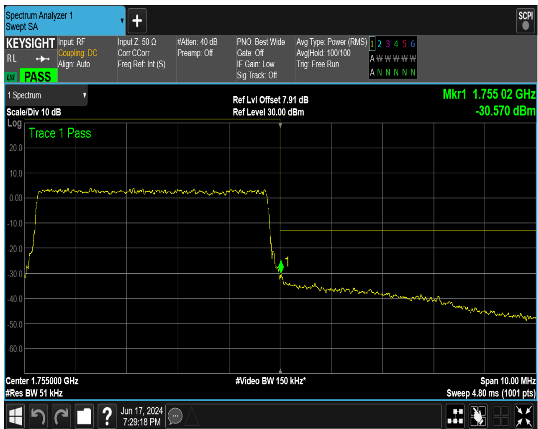
Band4 QPSK BW=1.4MHz Channel=19957 RB Size=6 Position=#0
