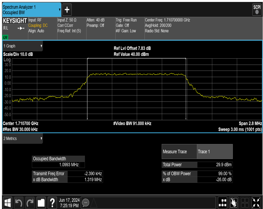
Band4 QAM16 BW=1.4MHz Channel=20175 RB Size=6 Position=#0
