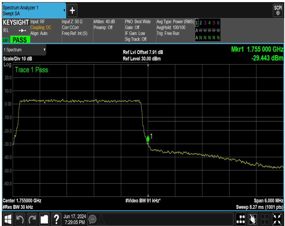
Band4 QAM16 BW=5MHz Channel=19975 RB Size=25 Position=#0
