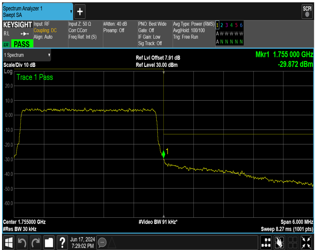
Band4 QPSK BW=5MHz Channel=19975 RB Size=25 Position=#0
