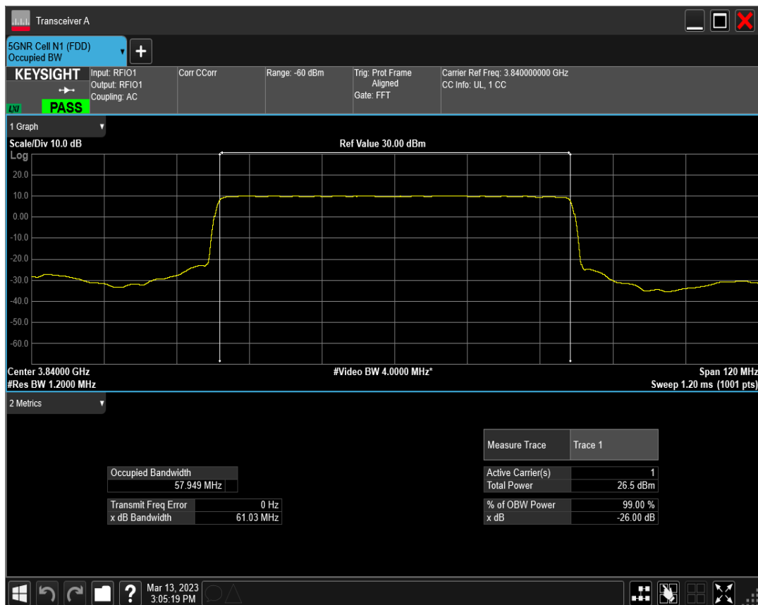
n77(3700-3980) SCS=30kHz DFT_QPSK BW=60MHz Channel=656000 RB=162@0
