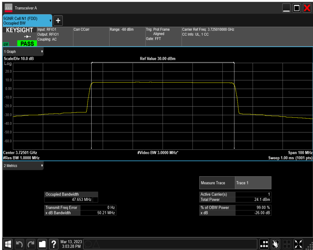
n77(3700-3980) SCS=30kHz DFT_BPSK BW=50MHz Channel=656000 RB=128@0
