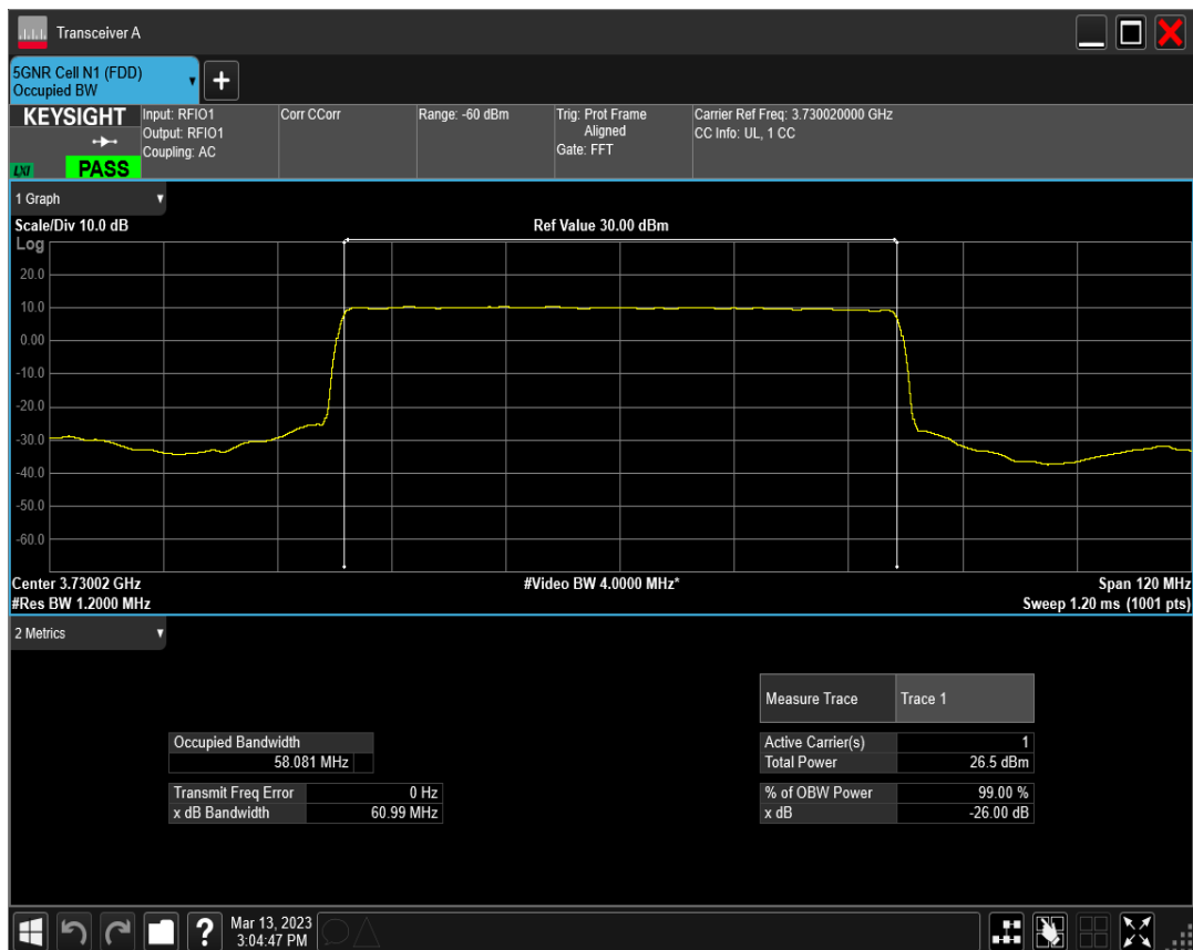
n77(3700-3980) SCS=30kHz DFT_QPSK BW=60MHz Channel=648668 RB=162@0
