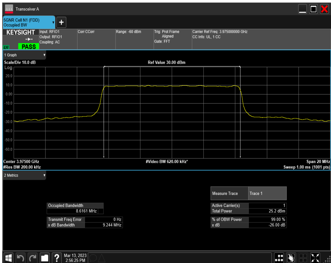
n77(3700-3980) SCS=30kHz DFT_QAM64 BW=10MHz Channel=665000 RB=24@0
