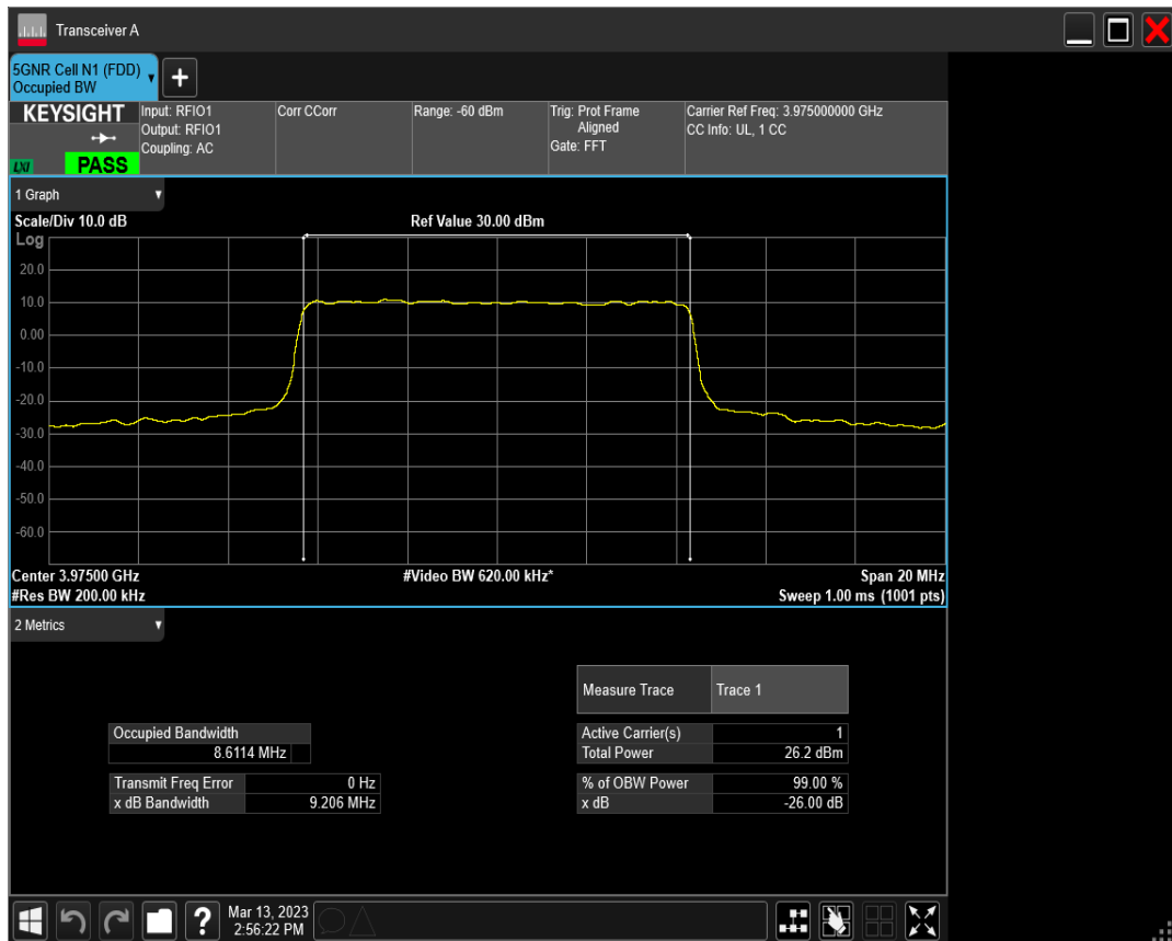
n77(3700-3980) SCS=30kHz DFT_QAM16 BW=10MHz Channel=665000 RB=24@0
