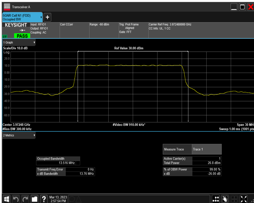
n77(3700-3980) SCS=30kHz DFT_QPSK BW=15MHz Channel=664832 RB=36@0
