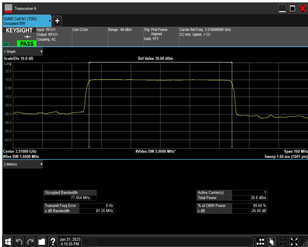
n77(3450-3550) SCS=30kHz DFT_QPSK BW=80MHz Channel=634000 RB=216@0
