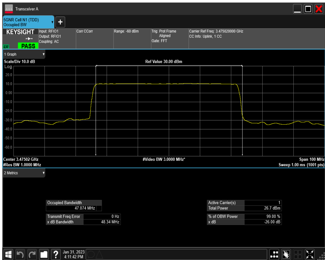
n77(3450-3550) SCS=30kHz DFT_QPSK BW=50MHz Channel=631668 RB=128@0
