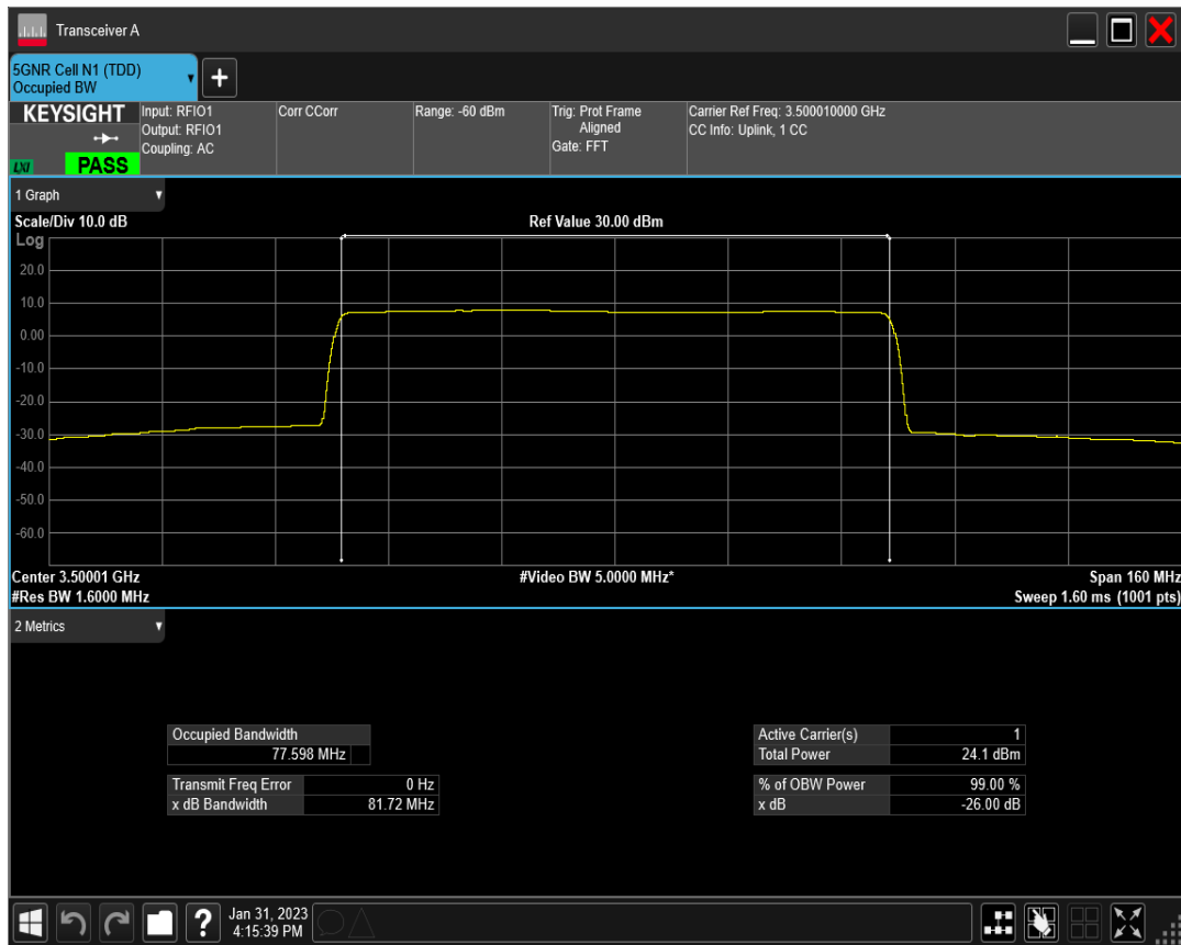
n77(3450-3550) SCS=30kHz DFT_BPSK BW=80MHz Channel=634000 RB=216@0
