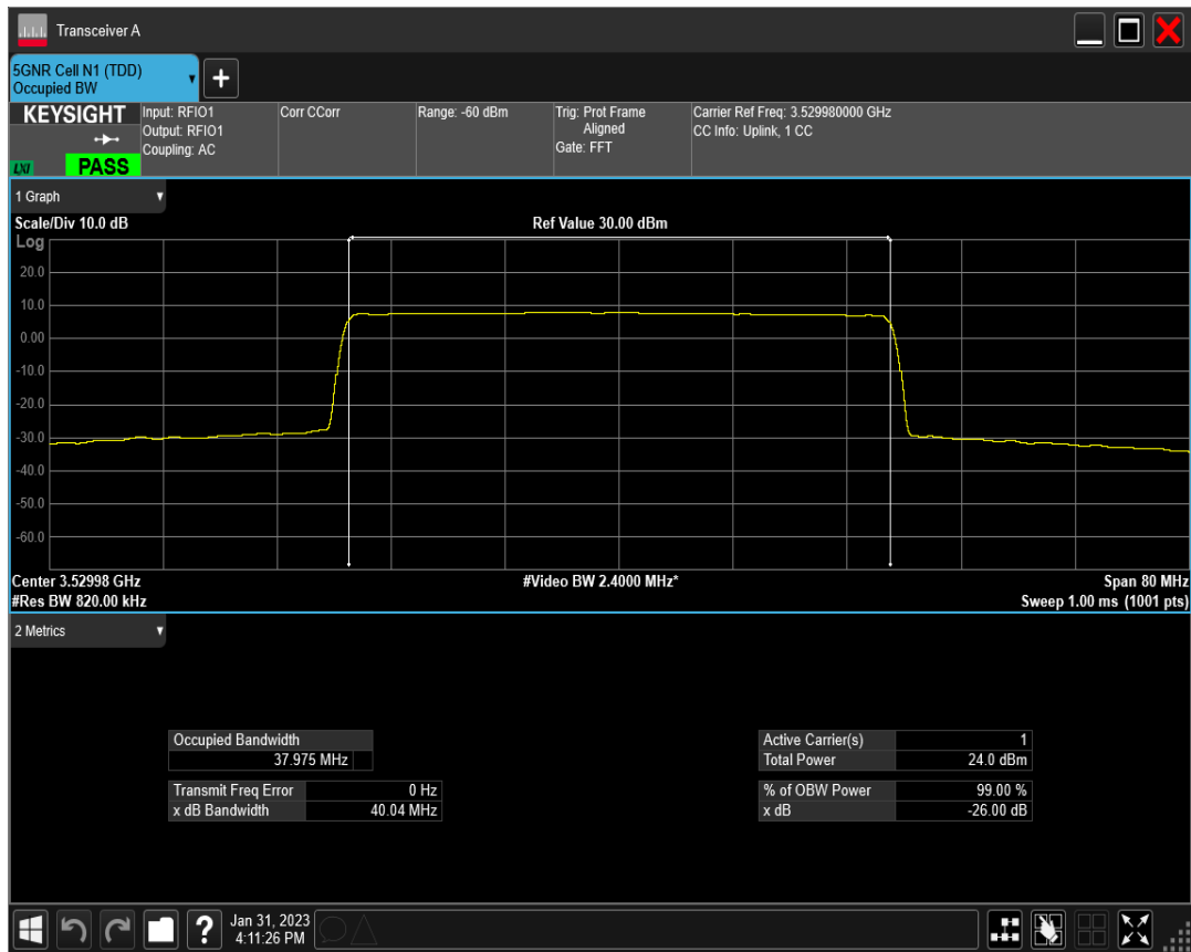
n77(3450-3550) SCS=30kHz DFT_BPSK BW=50MHz Channel=631668 RB=128@0
