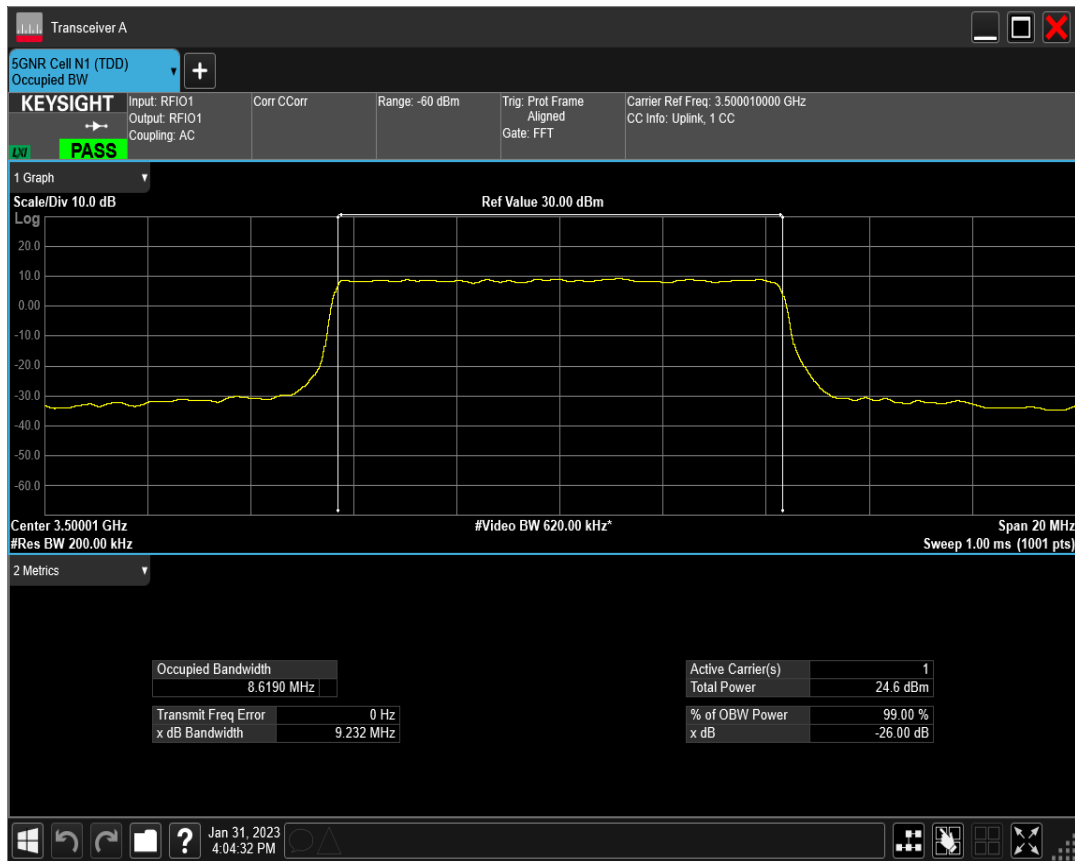
n77(3450-3550) SCS=30kHz DFT_QAM256 BW=10MHz Channel=633334 RB=24@0
