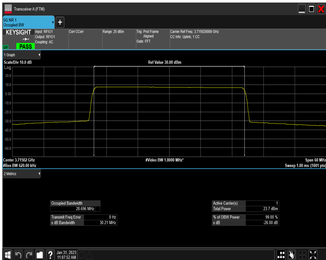
n77(3700-3980) SCS=15kHz DFT_BPSK BW=30MHz Channel=656000 RB=160@0
