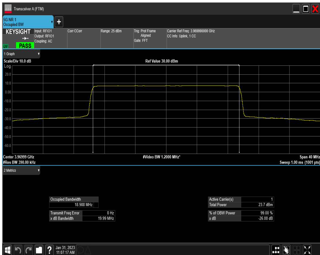
n77(3700-3980) SCS=15kHz DFT_BPSK BW=30MHz Channel=647668 RB=160@0
