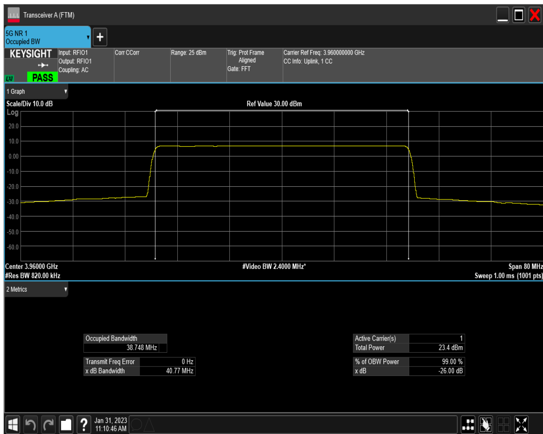
n77(3700-3980) SCS=15kHz DFT_BPSK BW=50MHz Channel=648334 RB=270@0
