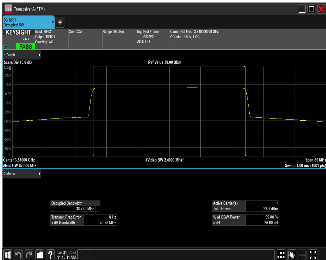
n77(3700-3980) SCS=15kHz DFT_BPSK BW=40MHz Channel=664000 RB=216@0
