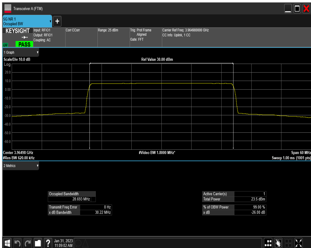
n77(3700-3980) SCS=15kHz DFT_BPSK BW=40MHz Channel=648000 RB=216@0
