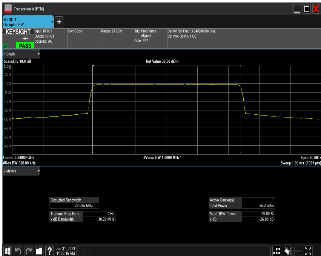
n77(3700-3980) SCS=15kHz DFT_QAM16 BW=30MHz Channel=656000 RB=160@0
