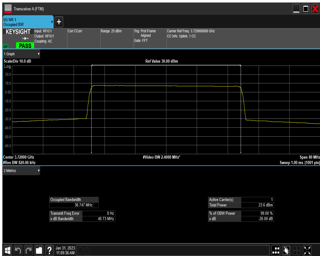
n77(3700-3980) SCS=15kHz DFT_BPSK BW=40MHz Channel=656000 RB=216@0
