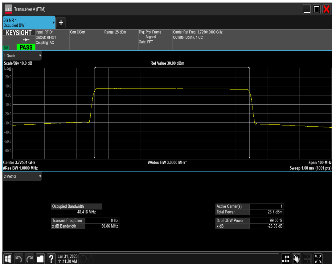
n77(3700-3980) SCS=15kHz DFT_BPSK BW=50MHz Channel=656000 RB=270@0
