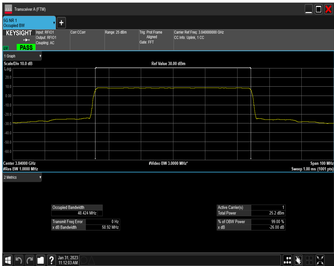
n77(3700-3980) SCS=15kHz DFT_BPSK BW=50MHz Channel=663666 RB=270@0
