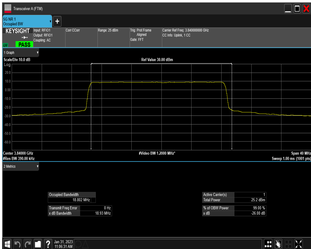
n77(3700-3980) SCS=15kHz DFT_QAM16 BW=20MHz Channel=656000 RB=100@0
