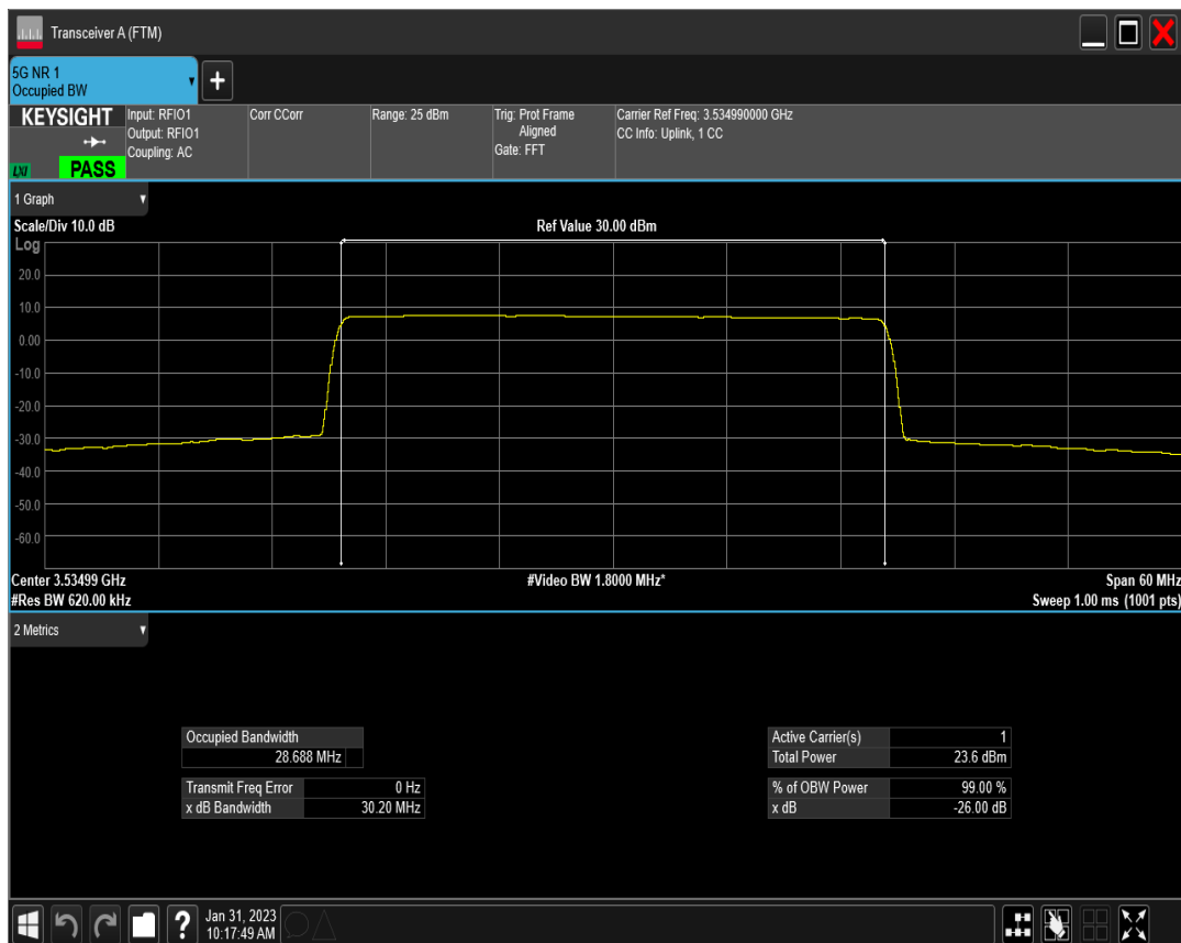
n77(3450-3550) SCS=15kHz DFT_BPSK BW=40MHz Channel=631334 RB=216@0
