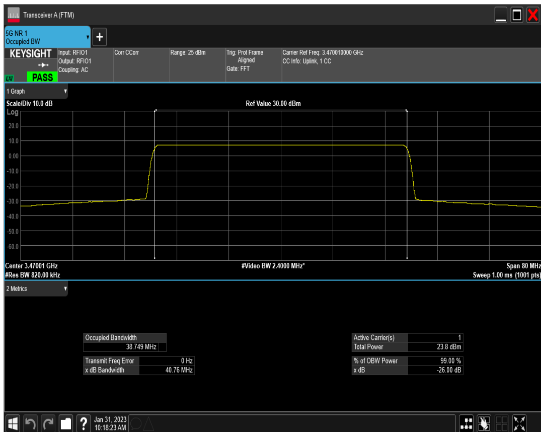
n77(3450-3550) SCS=15kHz DFT_BPSK BW=40MHz Channel=633334 RB=216@0
