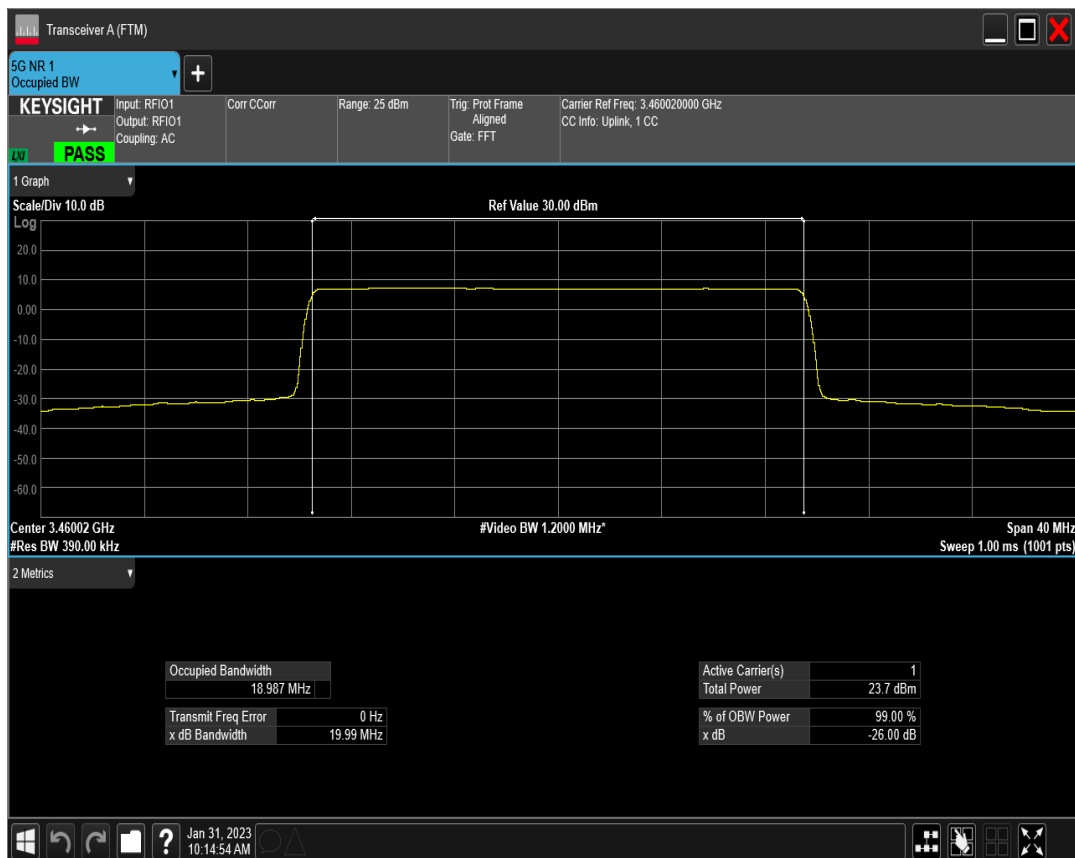
n77(3450-3550) SCS=15kHz DFT_BPSK BW=20MHz Channel=633334 RB=100@0
