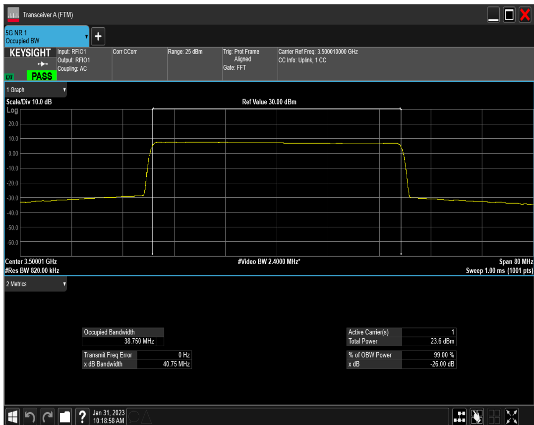
n77(3450-3550) SCS=15kHz DFT_BPSK BW=40MHz Channel=635332 RB=216@0
