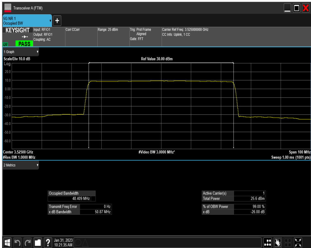
n77(3450-3550) SCS=15kHz DFT_QAM16 BW=50MHz Channel=635000 RB=270@0
