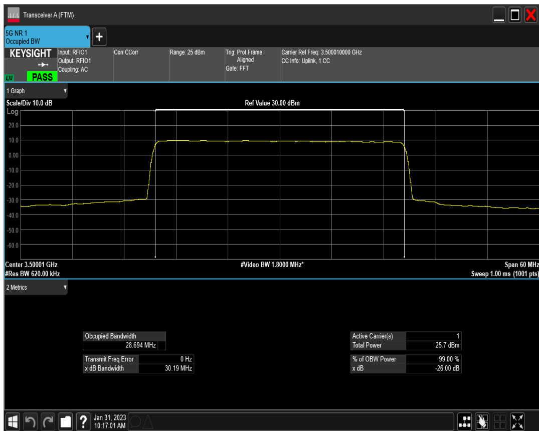
n77(3450-3550) SCS=15kHz DFT_QAM16 BW=30MHz Channel=633334 RB=160@0
