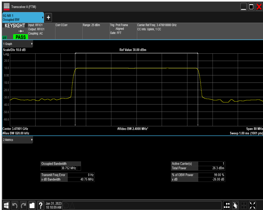
n77(3450-3550) SCS=15kHz DFT_QPSK BW=40MHz Channel=631334 RB=216@0
