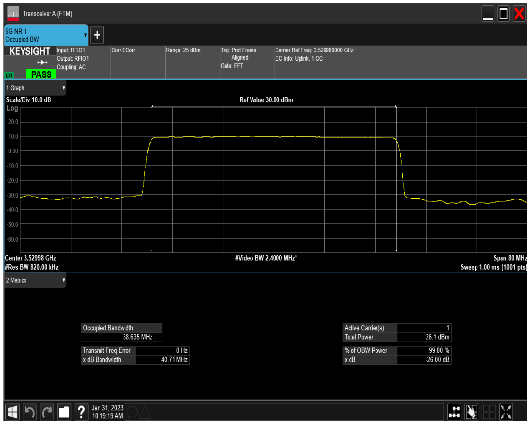
n77(3450-3550) SCS=15kHz DFT_QPSK BW=40MHz Channel=635332 RB=216@0
