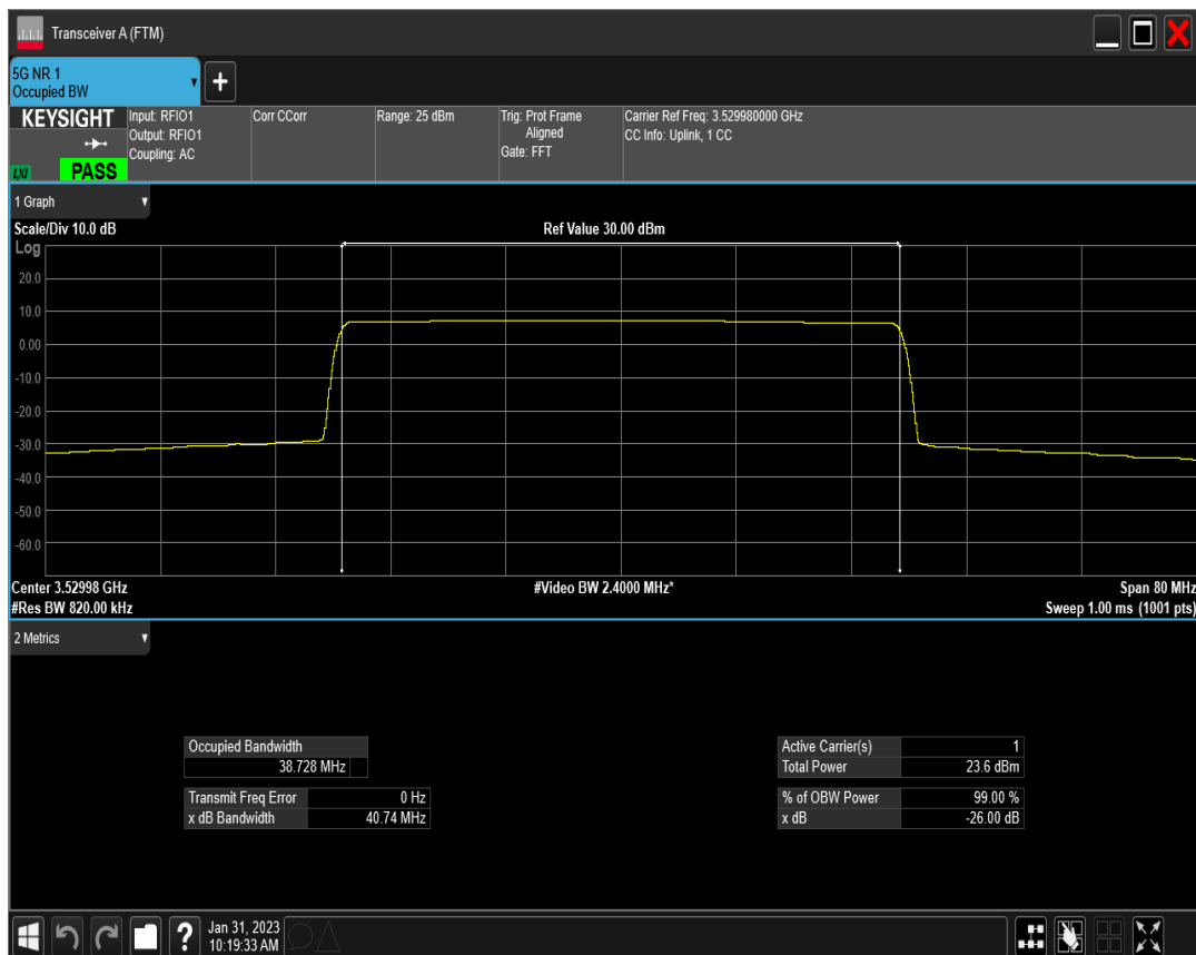
n77(3450-3550) SCS=15kHz DFT_BPSK BW=50MHz Channel=631668 RB=270@0
