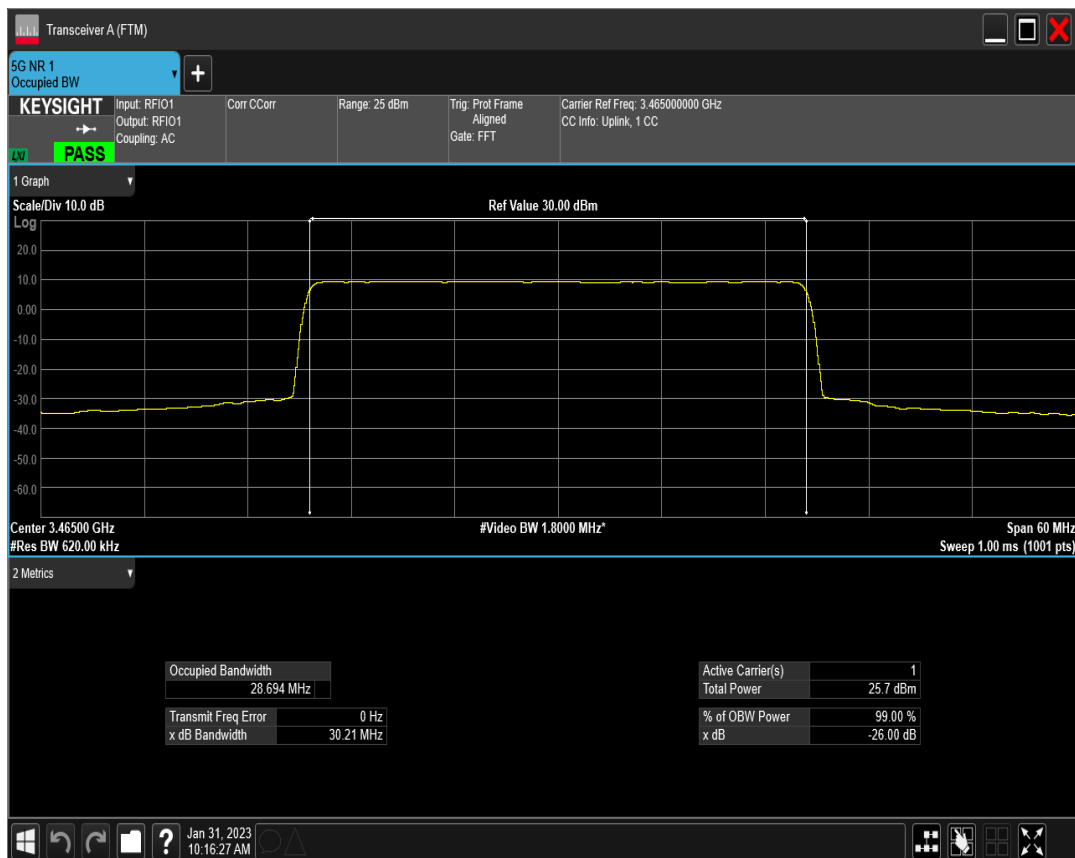
n77(3450-3550) SCS=15kHz DFT_QAM16 BW=30MHz Channel=631000 RB=160@0
