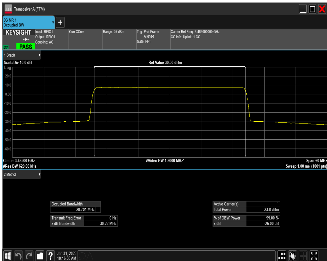
n77(3450-3550) SCS=15kHz DFT_BPSK BW=30MHz Channel=633334 RB=160@0
