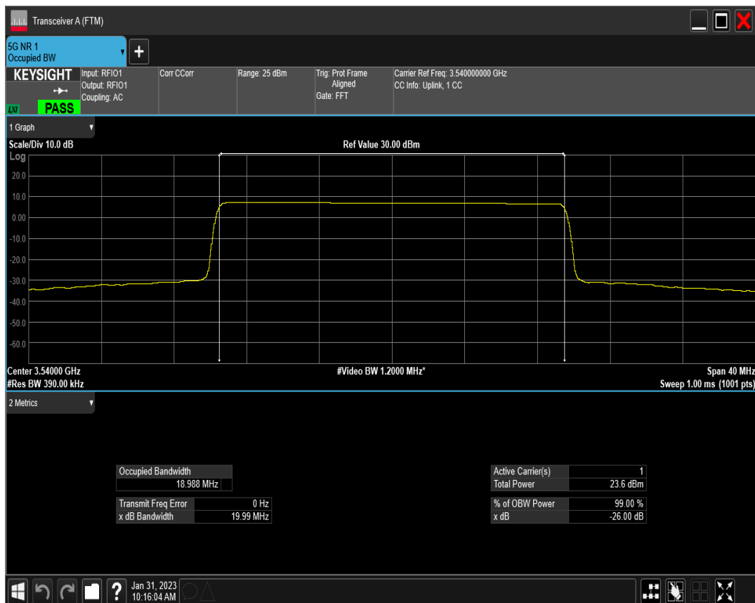
n77(3450-3550) SCS=15kHz DFT_BPSK BW=30MHz Channel=631000 RB=160@0
