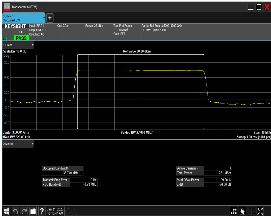
n77(3450-3550) SCS=15kHz DFT_QPSK BW=40MHz Channel=633334 RB=216@0
