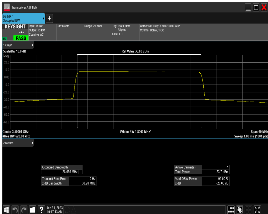
n77(3450-3550) SCS=15kHz DFT_BPSK BW=30MHz Channel=635666 RB=160@0
