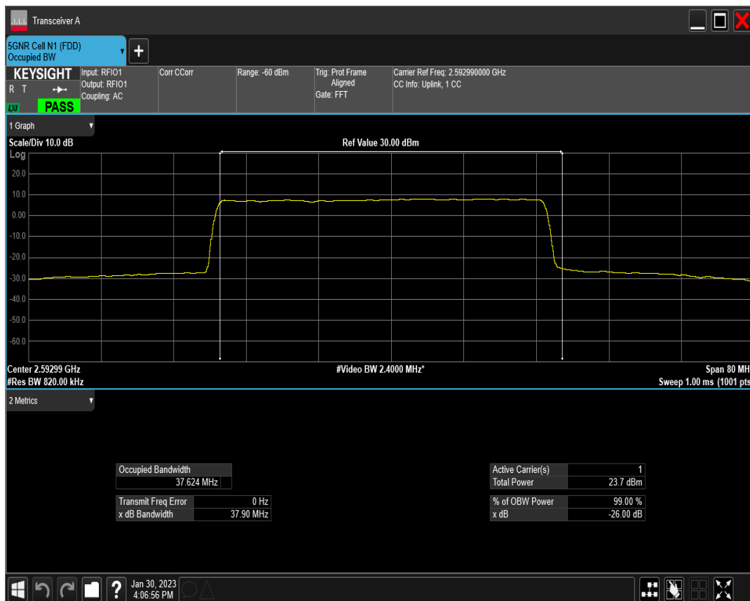
n41 SCS=30kHz DFT_QAM64 BW=40MHz Channel=518598 RB=100@0
