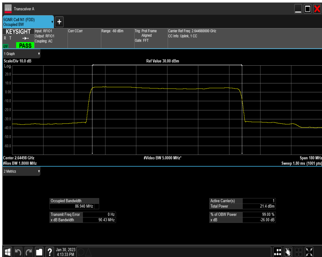
n41 SCS=30kHz CP_QPSK BW=90MHz Channel=528996 RB=245@0
