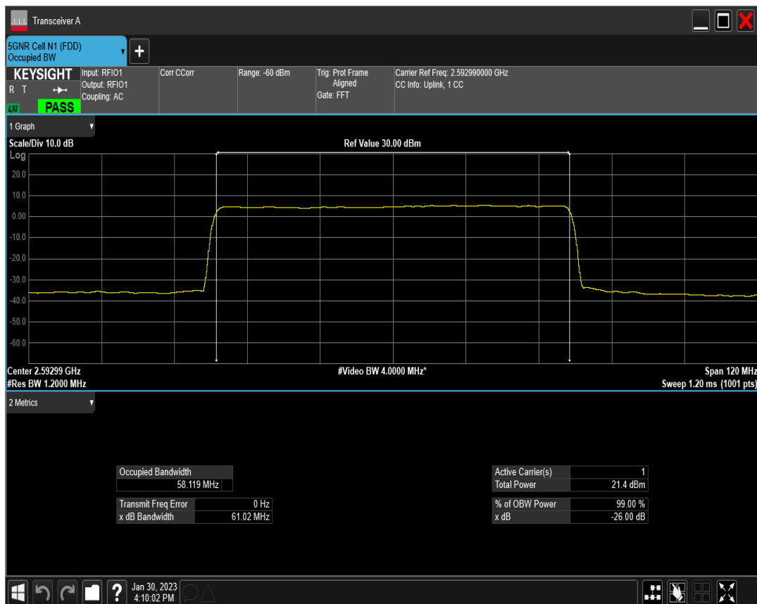
n41 SCS=30kHz CP_QPSK BW=60MHz Channel=518598 RB=162@0
