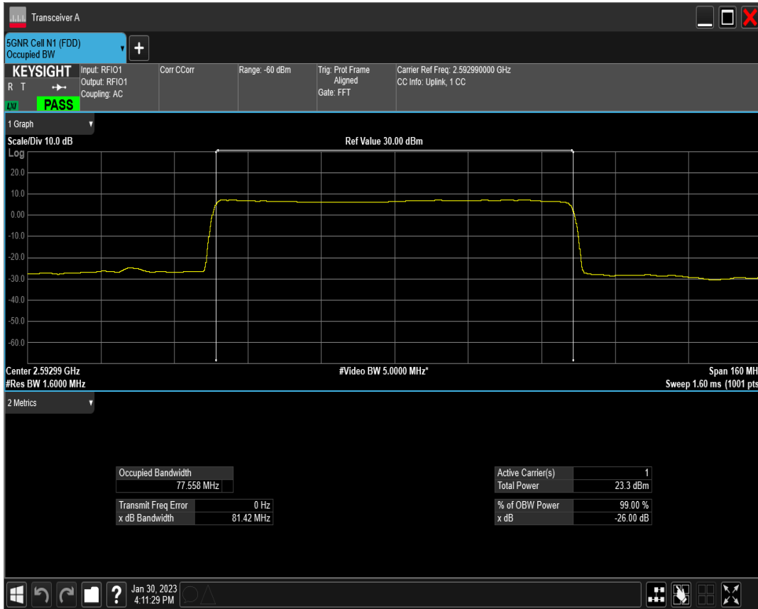
n41 SCS=30kHz DFT_QAM256 BW=80MHz Channel=518598 RB=216@0
