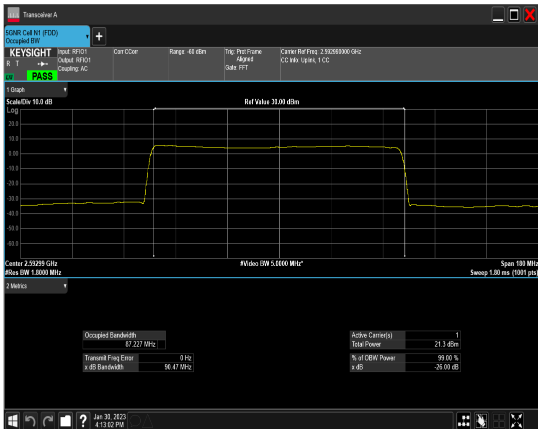
n41 SCS=30kHz CP_QPSK BW=90MHz Channel=518598 RB=245@0
