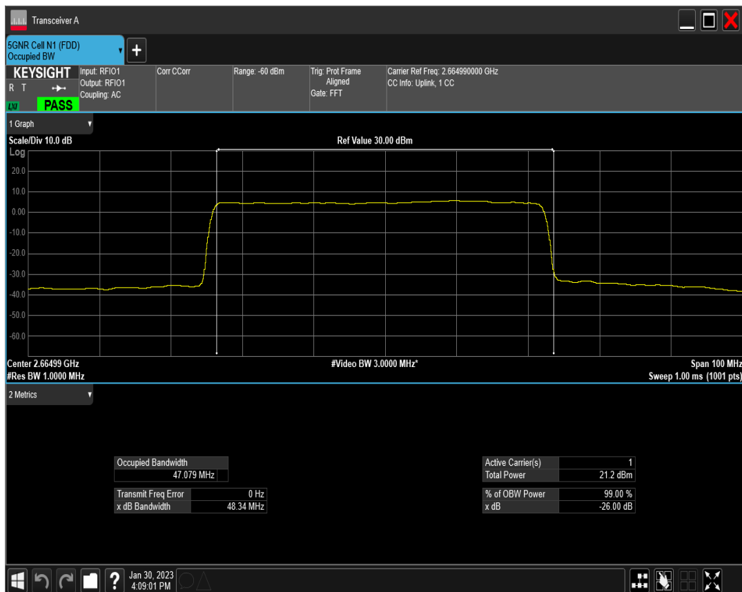
n41 SCS=30kHz CP_QPSK BW=50MHz Channel=532998 RB=133@0
