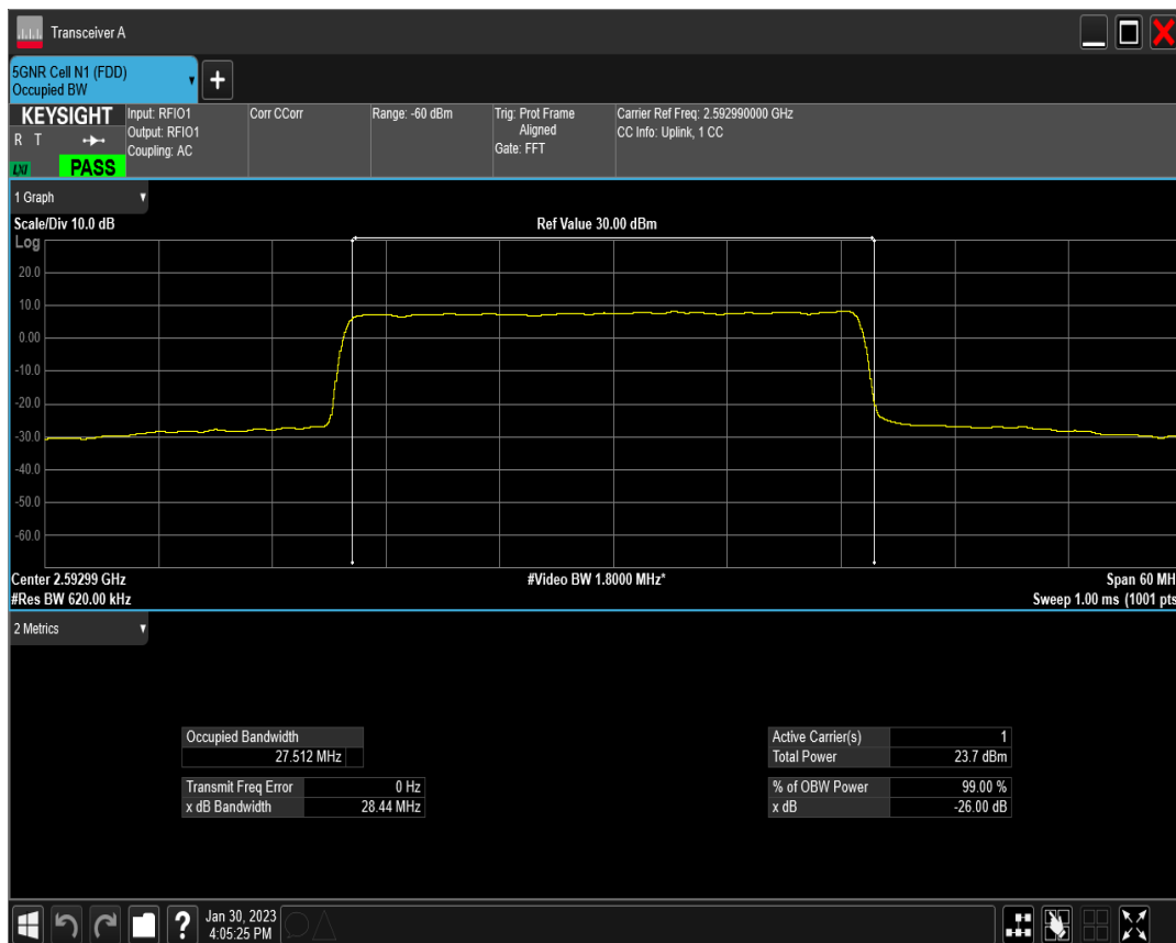
n41 SCS=30kHz DFT_QAM64 BW=30MHz Channel=518598 RB=75@0
