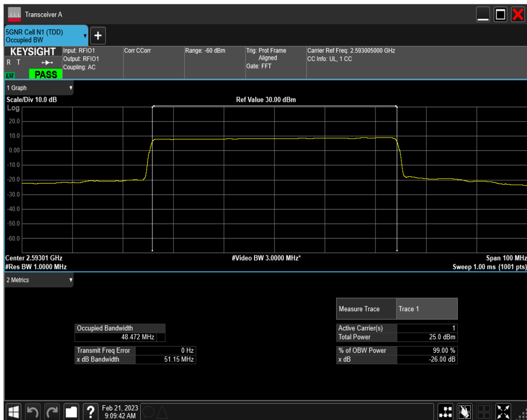
n41 SCS=15kHz DFT_QAM16 BW=50MHz Channel=518601 RB=270@0
