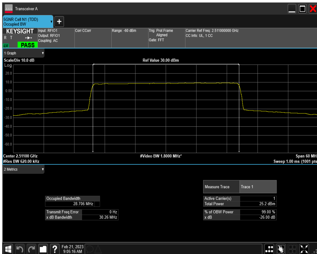
n41 SCS=15kHz DFT_QAM16 BW=30MHz Channel=502200 RB=160@0
