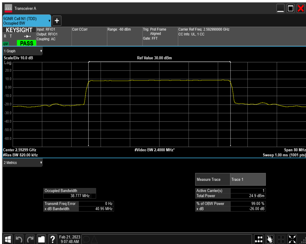
n41 SCS=15kHz DFT_QAM16 BW=40MHz Channel=518598 RB=216@0
