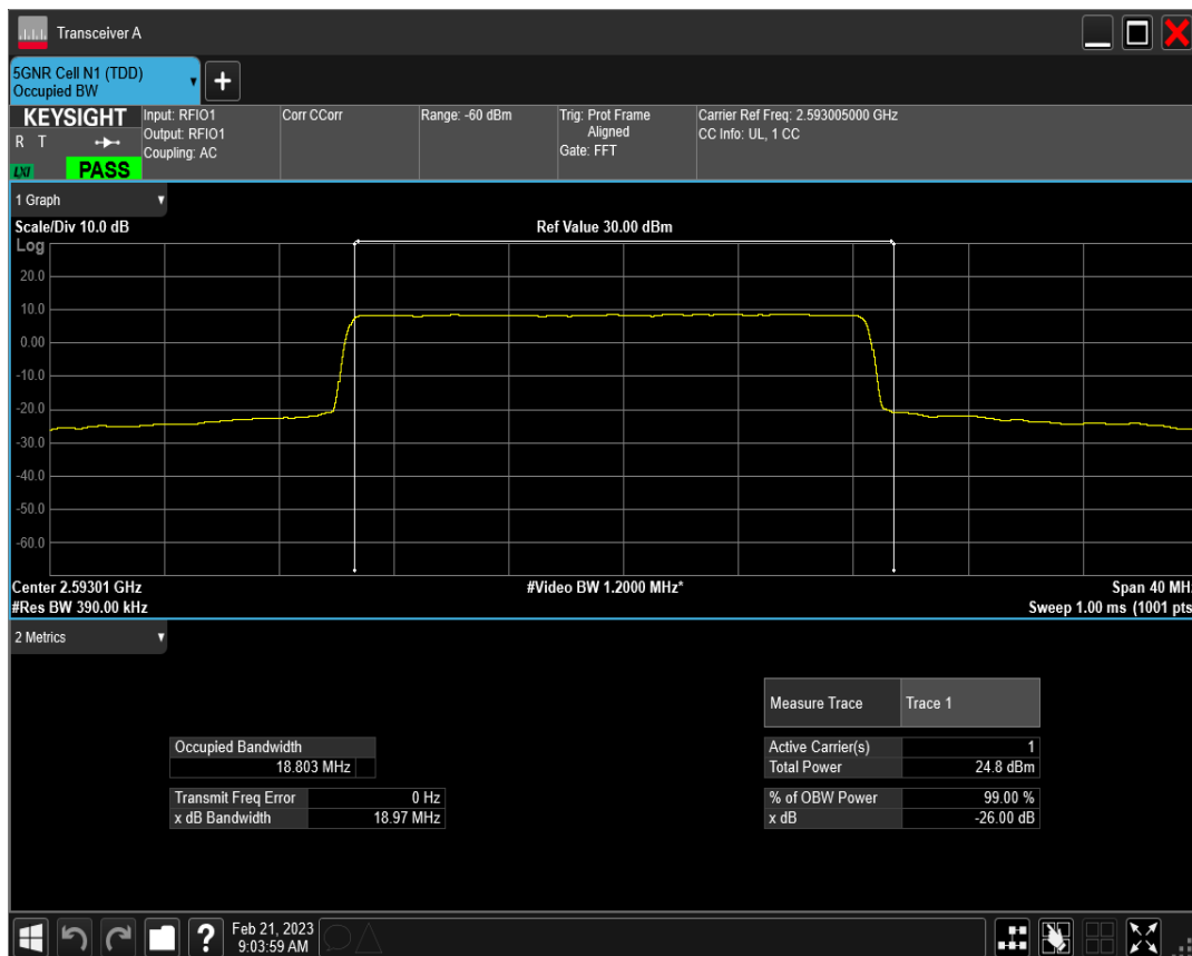
n41 SCS=15kHz DFT_QAM16 BW=20MHz Channel=518601 RB=100@0
