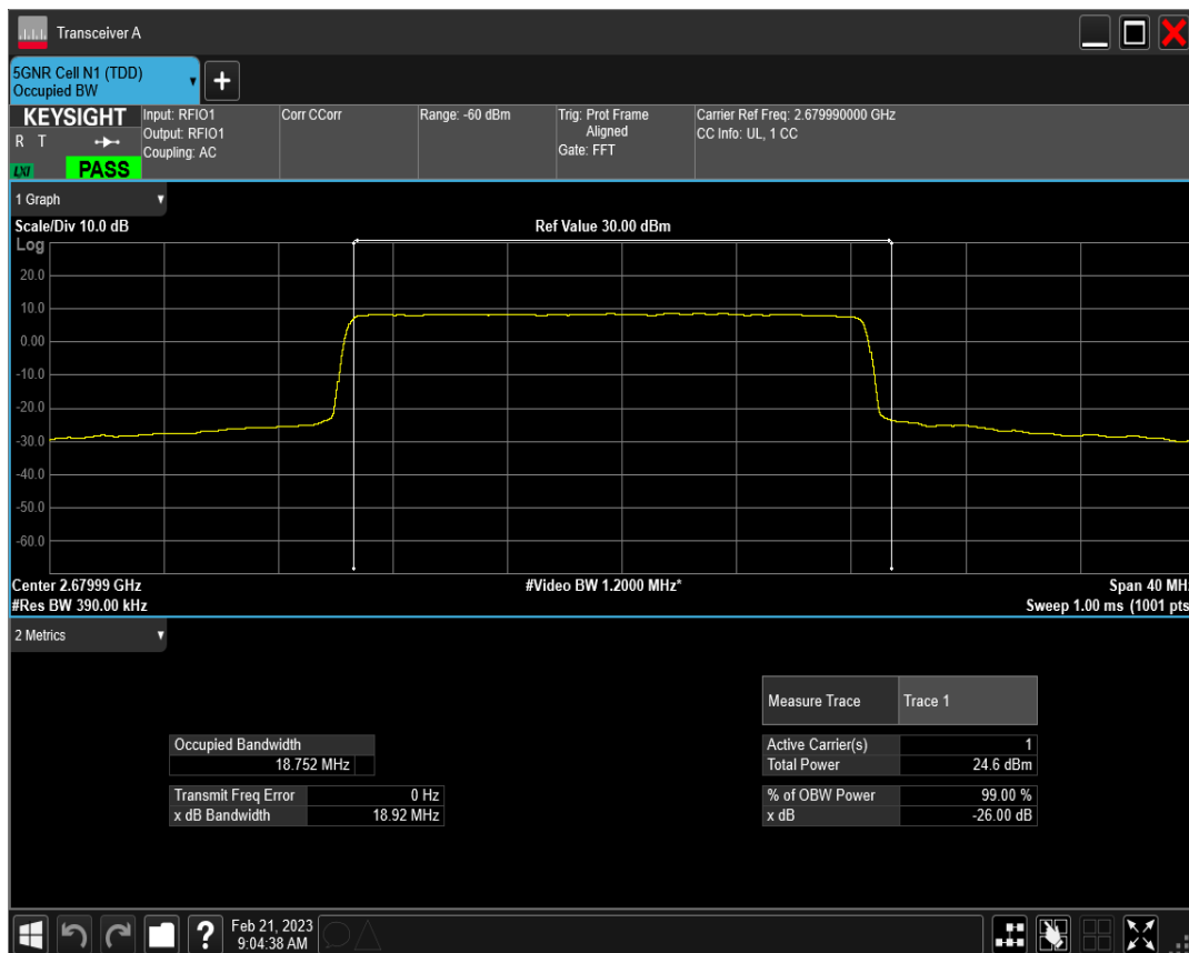
n41 SCS=15kHz DFT_QAM16 BW=20MHz Channel=535998 RB=100@0
