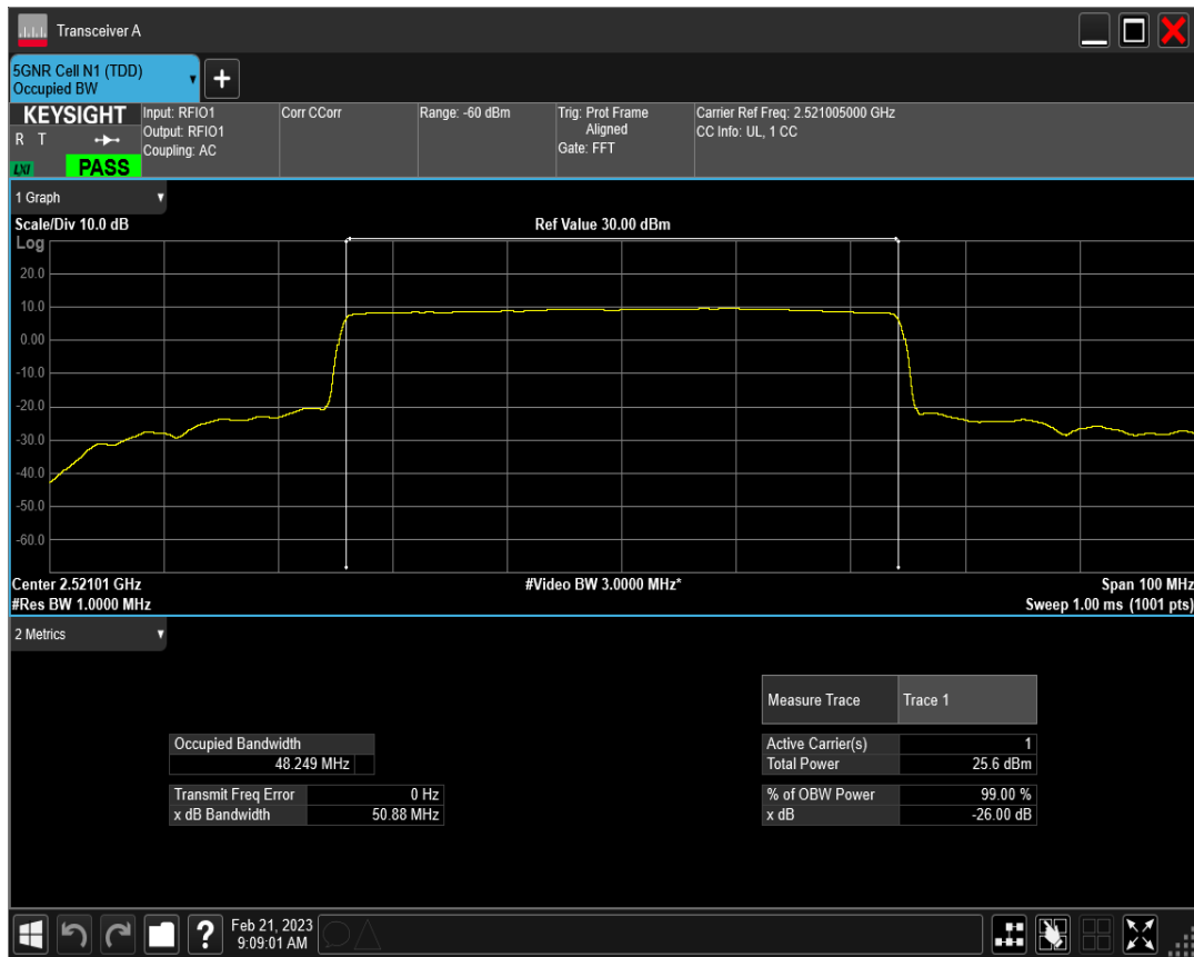
n41 SCS=15kHz DFT_QPSK BW=50MHz Channel=504201 RB=270@0
