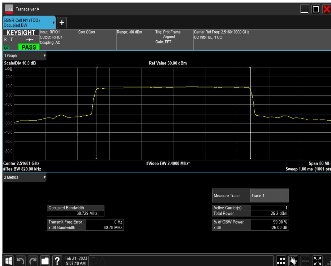
n41 SCS=15kHz DFT_QAM16 BW=40MHz Channel=503202 RB=216@0
