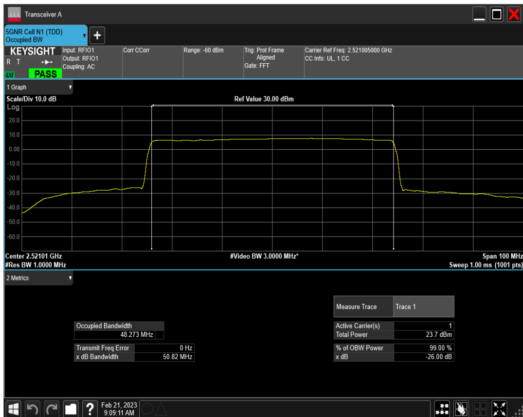
n41 SCS=15kHz DFT_QAM256 BW=50MHz Channel=504201 RB=270@0
