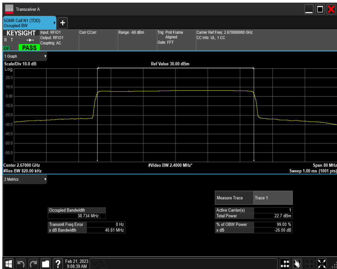
n41 SCS=15kHz DFT_BPSK BW=50MHz Channel=504201 RB=270@0
