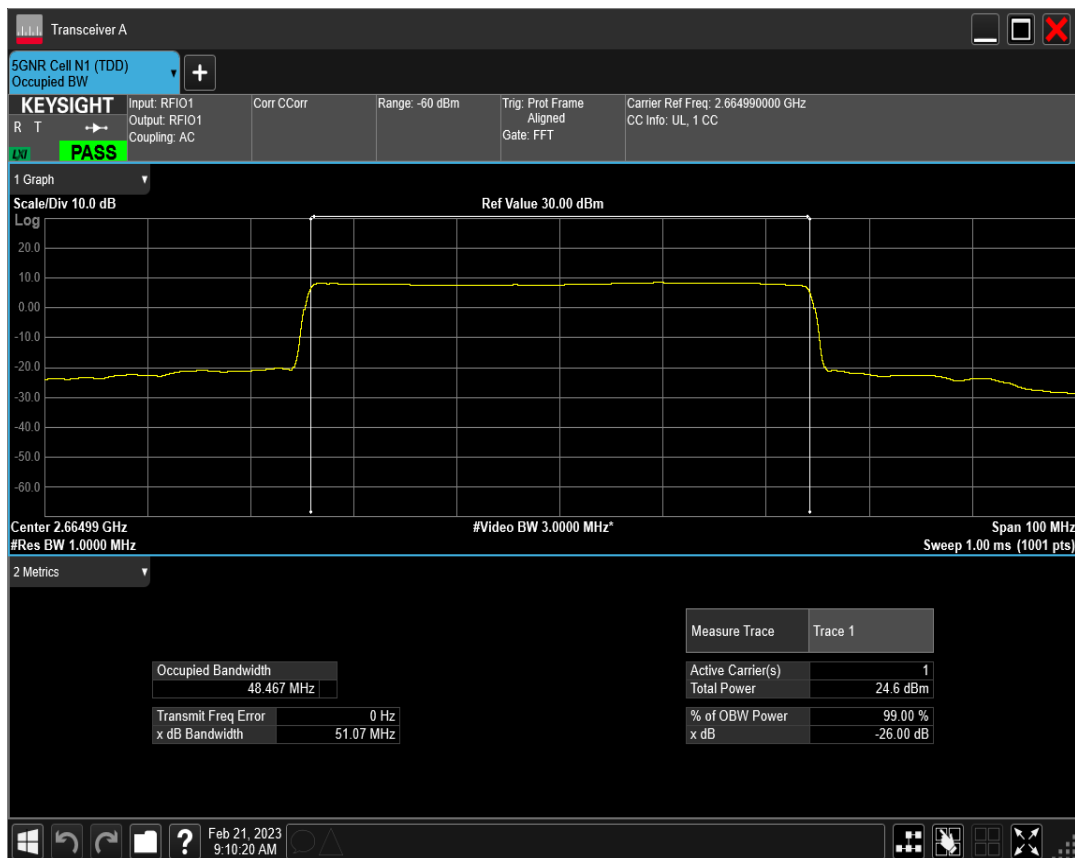
n41 SCS=15kHz DFT_QAM16 BW=50MHz Channel=532998 RB=270@0
