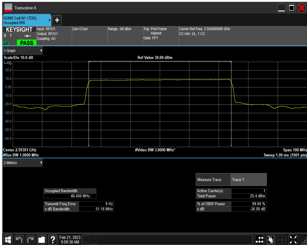
n41 SCS=15kHz DFT_QPSK BW=50MHz Channel=518601 RB=270@0
