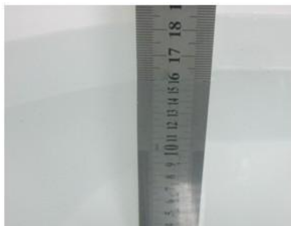
Liquid Height for Body SAR
