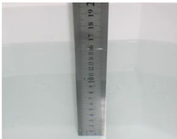
Liquid Height for Head SAR
