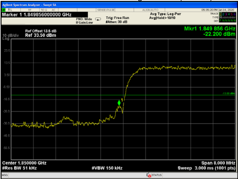
WCDMA band II band edge-left side (HSUPA)
