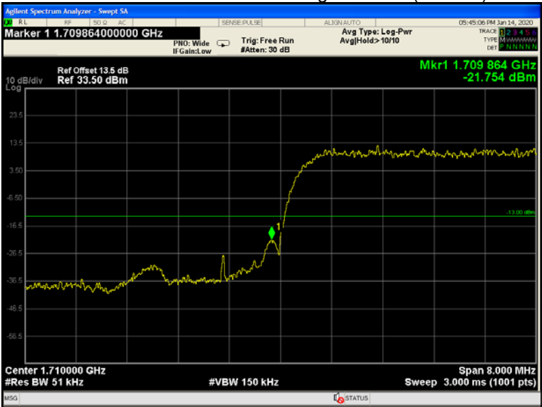
WCDMA band IV band edge-left side (HSUPA)
