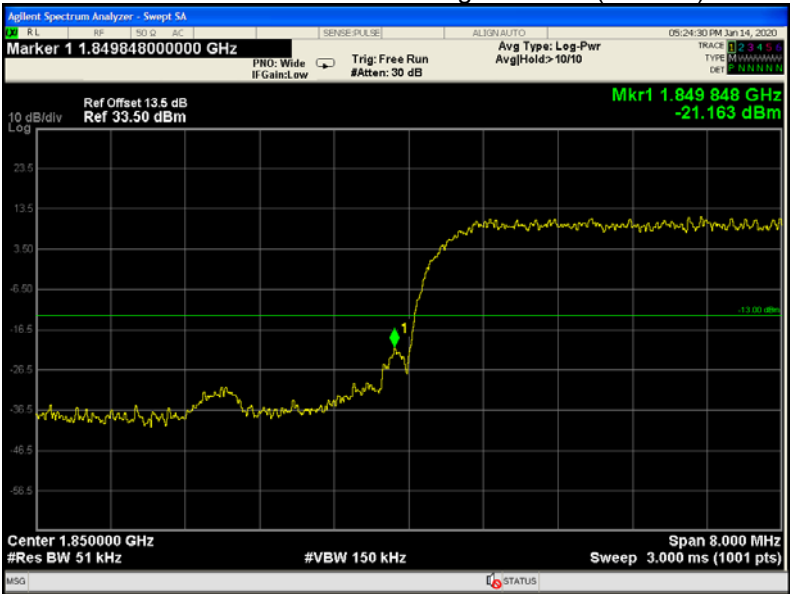
WCDMA band II band edge-left side (HSDPA)
