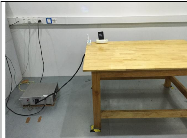
Conducted Emissions Test Setup Front View
