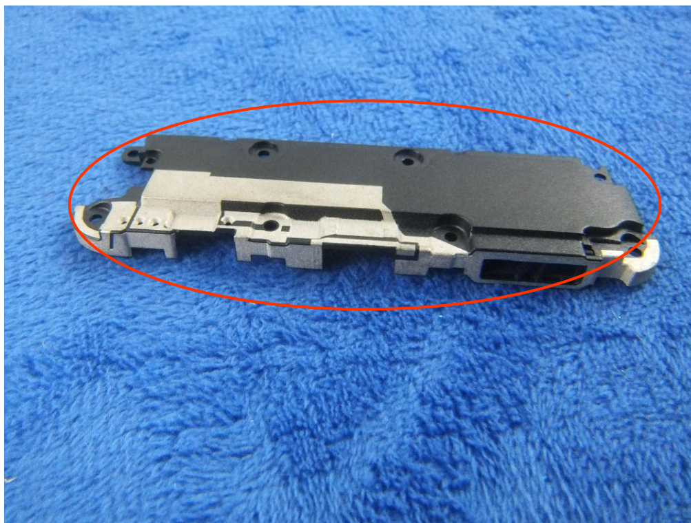
GSM/PCS/UMTS-FDD Antenna View
