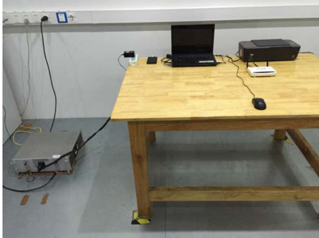
Conducted Emissions Test Setup – Front View
