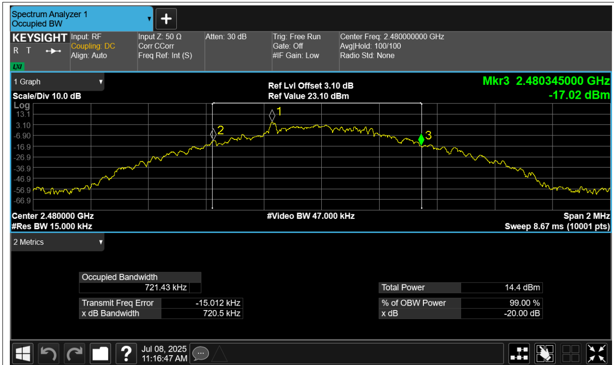
-20dB Bandwidth NVNT 2-DH1 2402MHz Ant3
