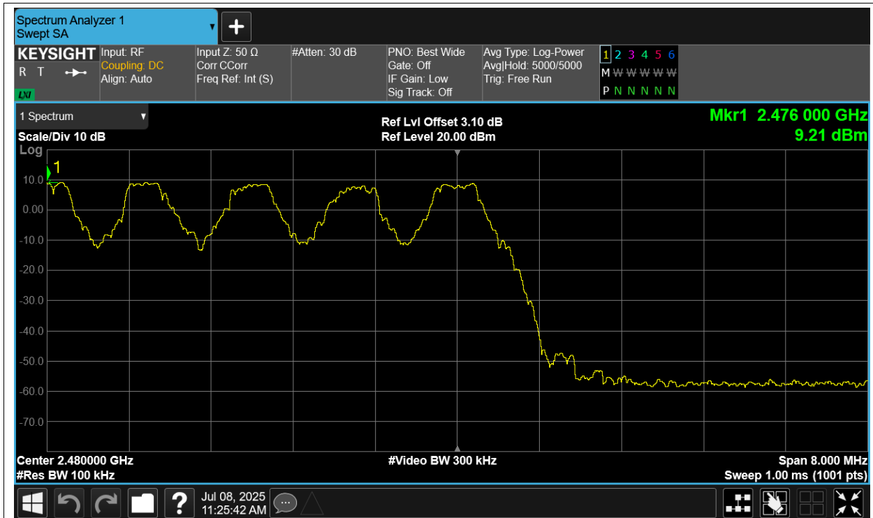
Band Edge(Hopping) NVNT 1-DH1 2480MHz Ant3 Hopping Emission
