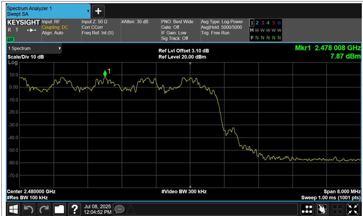
Band Edge(Hopping) NVNT 3-DH1 2480MHz Ant3 Hopping Emission
