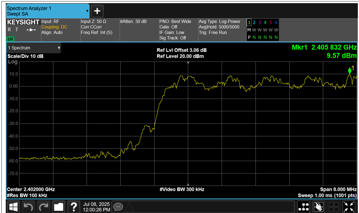
Band Edge(Hopping) NVNT 3-DH1 2402MHz Ant3 Hopping Emission
