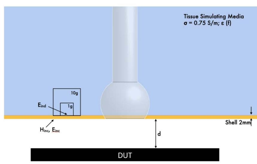
Distance used in the tables for simulation and compliance evaluation results is defined as the spacing between the top surface of the DUT and the bottom surface of the fictive phantom shell (with a thickness of 2mm). In this case, the evaluation is made at distance  $d$ . Typically  $d = 0$ , i.e., at the DUT surface. The evaluation locations of the incident fields (i.e.,  $H$  inc and  $E$  inc) as well as the induced fields (e.g.,  $E$  ind, psSAR1g, and psSAR10g) are also illustrated.
