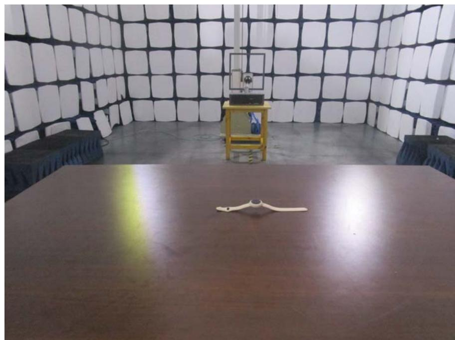
**Radiation Emission Test Setup (30MHz to 1GHz)**
