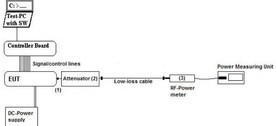
**Testing method:** ANSI C63.10:2013, KDB 558074 D01 DTS Meas.Guidance v03r05
