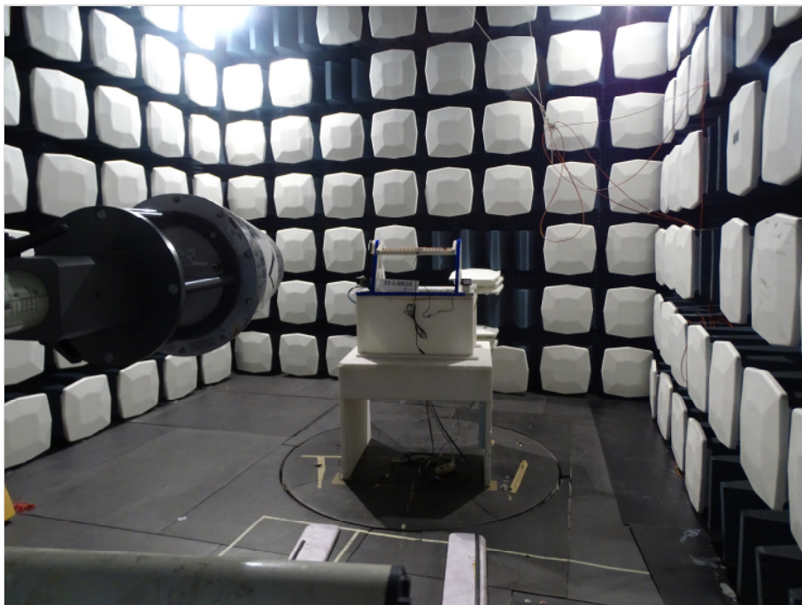
Photograph 4: EUT test setup in the fully anechoic chamber, overview_EUT elevation 0°
