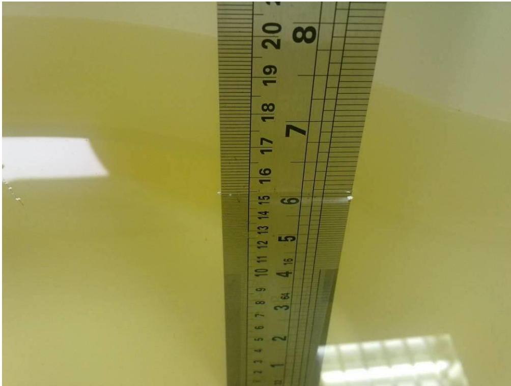
Photograph of the depth in the Phantom (850MHz)
