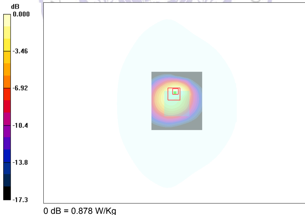
Figure 2: Wrist-Worn (GSM850 Middle Channel)
