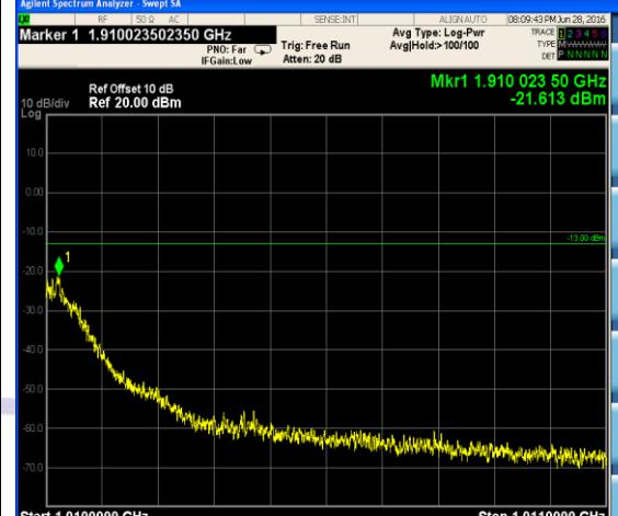
Start 1.9100000 GHz #Res BW 3.0 kHz #VBW 30 kHz Stop 1.9110000 GHz Sweep 103 ms (10000 pts)
