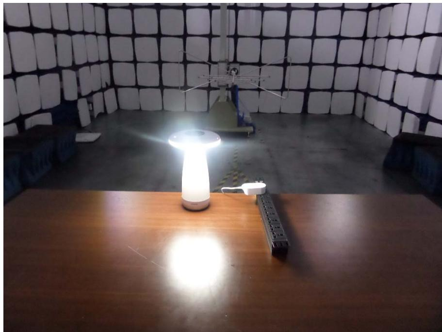
**Radiation Emission Test Setup (Above 1GHz)**
