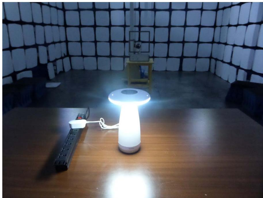
**Radiation Emission Test Setup (30MHz to 1GHz)**
