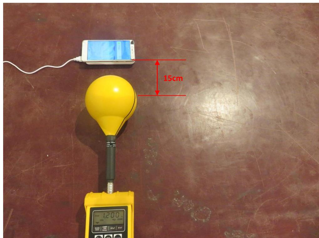
DUT – measurement position E – front side with 20 cm distance charging smartphone (SAMSUNG Galaxy S7)
