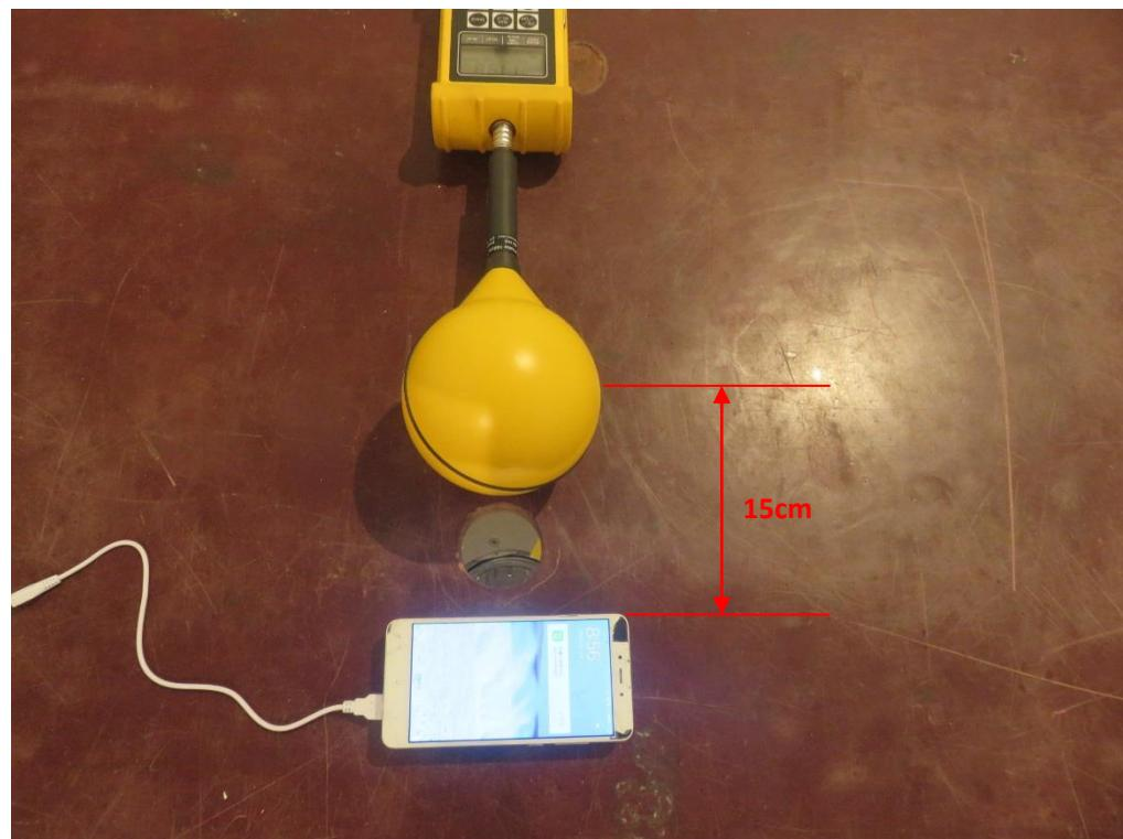
DUT – measurement position C – bottom side with 15 cm distance charging smartphone (SAMSUNG Galaxy S7)
