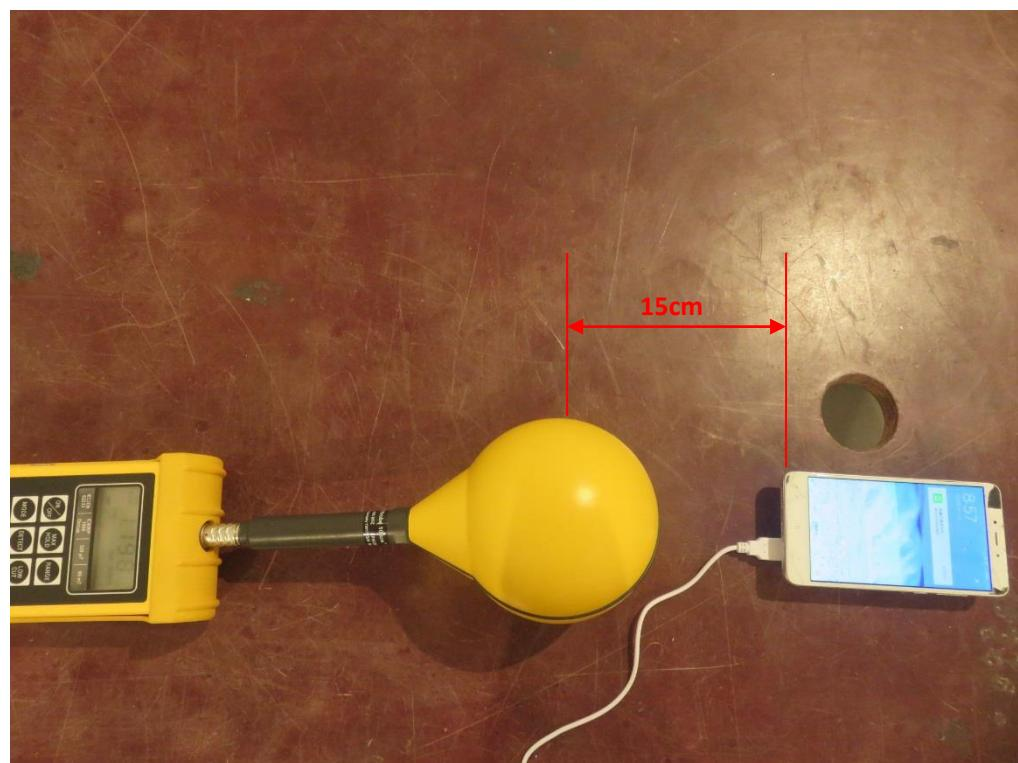
DUT – measurement position D – right side with 15 cm distance charging smartphone (SAMSUNG Galaxy S7)
