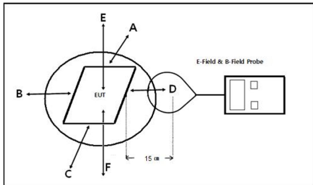
Due to installation limitations no tests from the underside of the charging device (Test Position F) are required.
