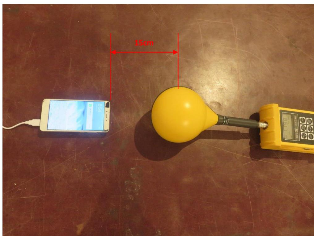
DUT – measurement position B – left side with 15 cm distance charging smartphone (SAMSUNG Galaxy S7)
