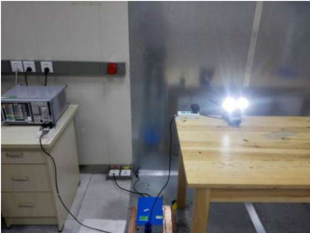
FCC RADIATED EMISSION TEST SETUP BELOW 1GHZ
