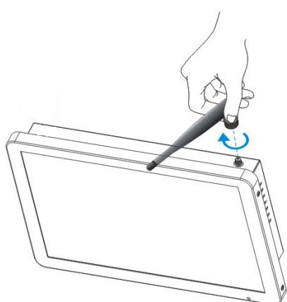
Use a clockwise motion to connect the antenna.
