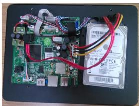
4. Fix HDD to the device mid-plate with screws.
