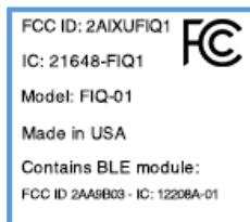
The FCC ID is displayed when the device is powered-on. The device can be powered on by pressing & holding the button on the tag for 6 seconds, then pressing again.
