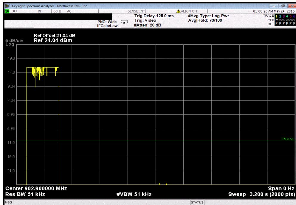
Hopping Mode, Mid Channel 902.9 MHz, 5470bps (Spreading Factor 7) OBW 125KHz, Pulse Width
