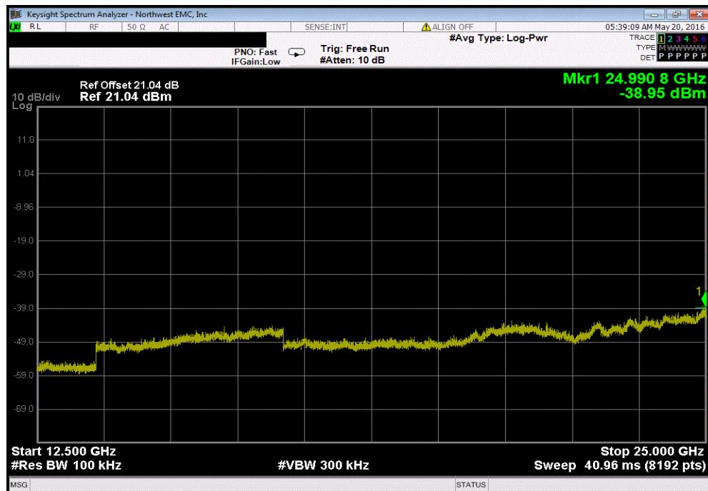
Non Hopping Mode, 5470bps (Spreading Factor 7) OBW 125KHz, High Channel, 903.7 MHz
