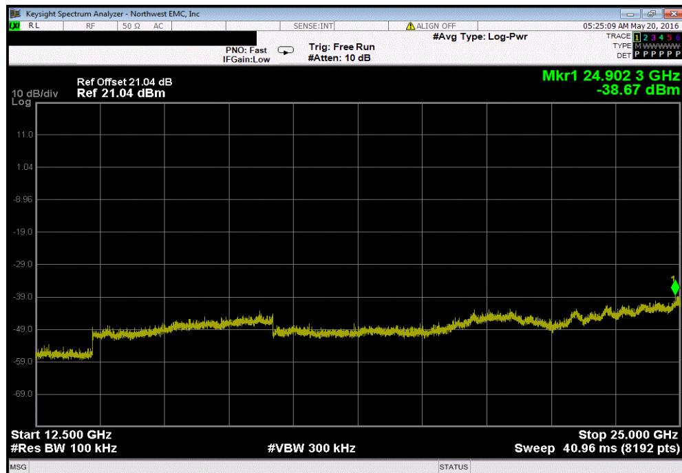
Non Hopping Mode, 980bps (Spreading Factor 10) OBW 125KHz, High Channel, 903.7 MHz
