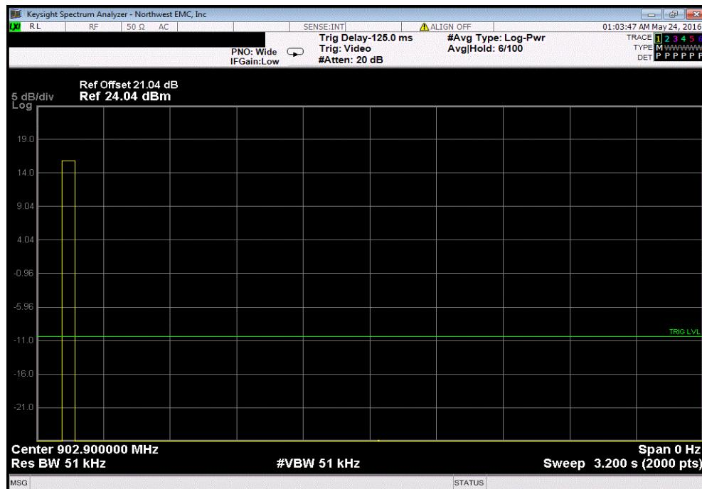
Hopping Mode, Mid Channel 902.9 MHz, 5470bps (Spreading Factor 7) OBW 125KHz, Sample 4
