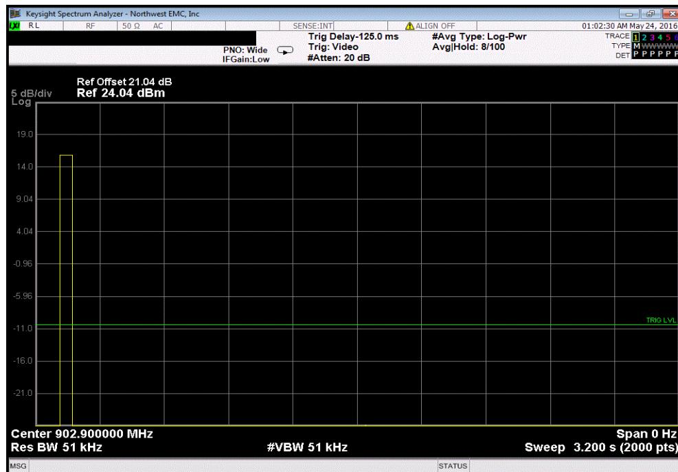
Hopping Mode, Mid Channel 902.9 MHz, 5470bps (Spreading Factor 7) OBW 125KHz, Sample 2
