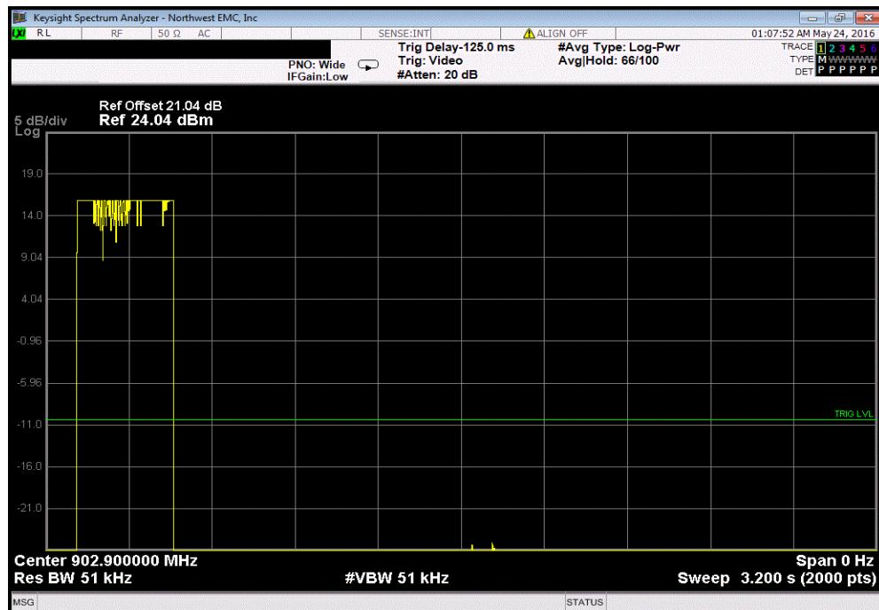
Hopping Mode, Mid Channel 902.9 MHz, 980bps (Spreading Factor 10) OBW 125KHz, Sample 3
