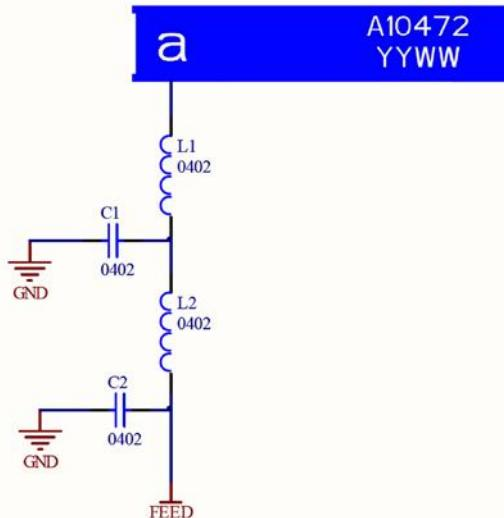
Note: The component values for the matching circuit will vary depending on the size of the PCB and surrounding components. The impedance of the antenna should be measured before selecting suitable matching components. Antenova M2M offers this service on request. Contact [sales@antenova-m2m.com](mailto:sales@antenova-m2m.com) for further information.
