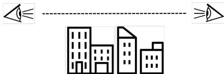
Because the link distances are usually within 10 km obstructions in the path can easily be identified using binoculars. It is important to understand that the Line-of-Sight is not just a thin line but more closely resembles a cone. To avoid signal degradation within the First Fresnel Zone, no obstacles should be located within a 1-4.5 meter (1.2-14.7 ft.) radius around the center axis of the Line-of-Sight.
