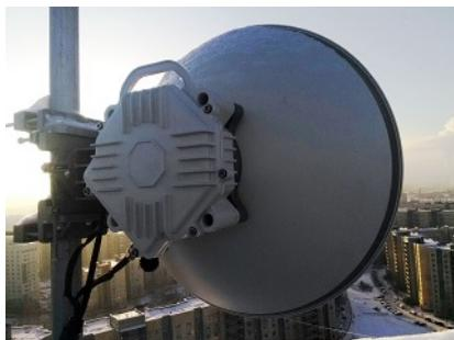
The PPC-10G wireless link is intended for full duplex 10 Gigabit Ethernet radio communication between two locations. It is comprised of two subscriber transceivers, each operating under line-of-sight conditions at working frequencies within the 71/86 GHz or 40.5-43.5GHz radio bands.
