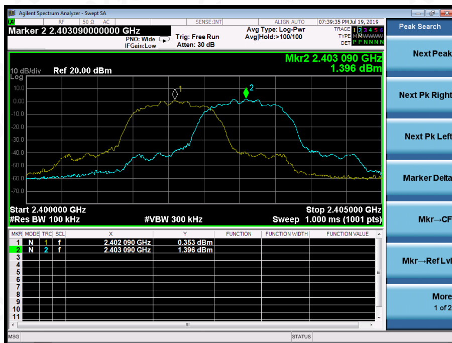
TEST PLOT FOR FREQUENCY SEPARATION
