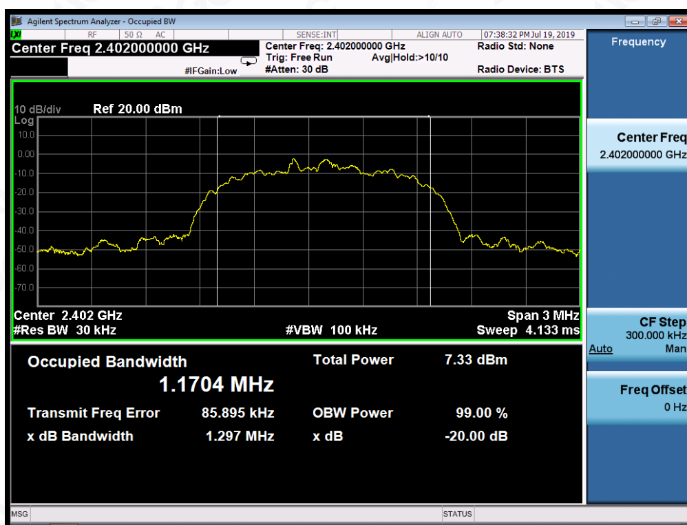
TEST PLOT OF BANDWIDTH FOR LOW CHANNEL
