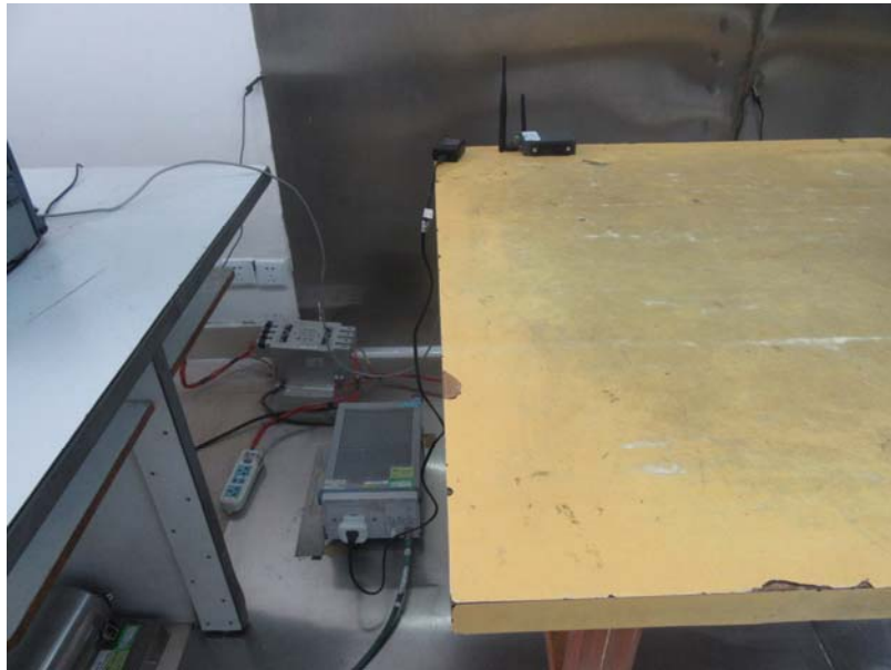
Conducted Emission Test Setup Front View
