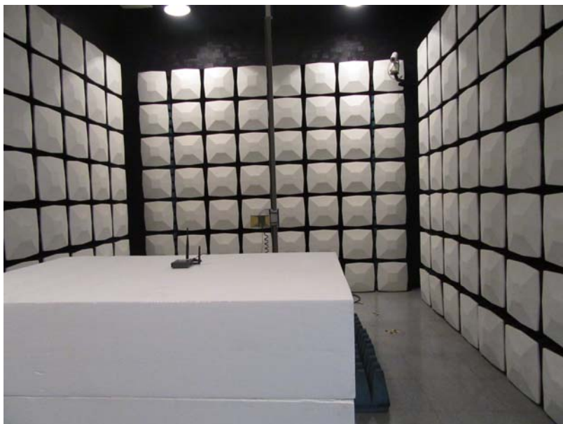
Radiated Emission Test Setup View (Above 1 GHz)
