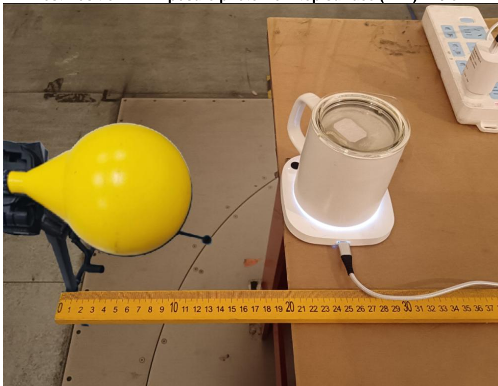
Test Position A - Exposure photo from top surface (TM1) - 20 cm
