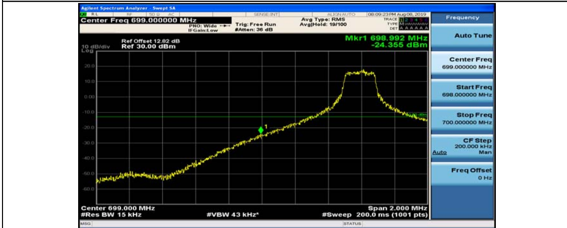
Channel Bandwidth: 10 MHz_LCH_16QAM_1RB#24
