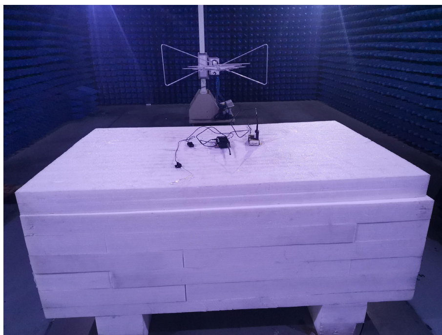
Photo of Radiated Emission Measurement (30MHz-1GHz)
