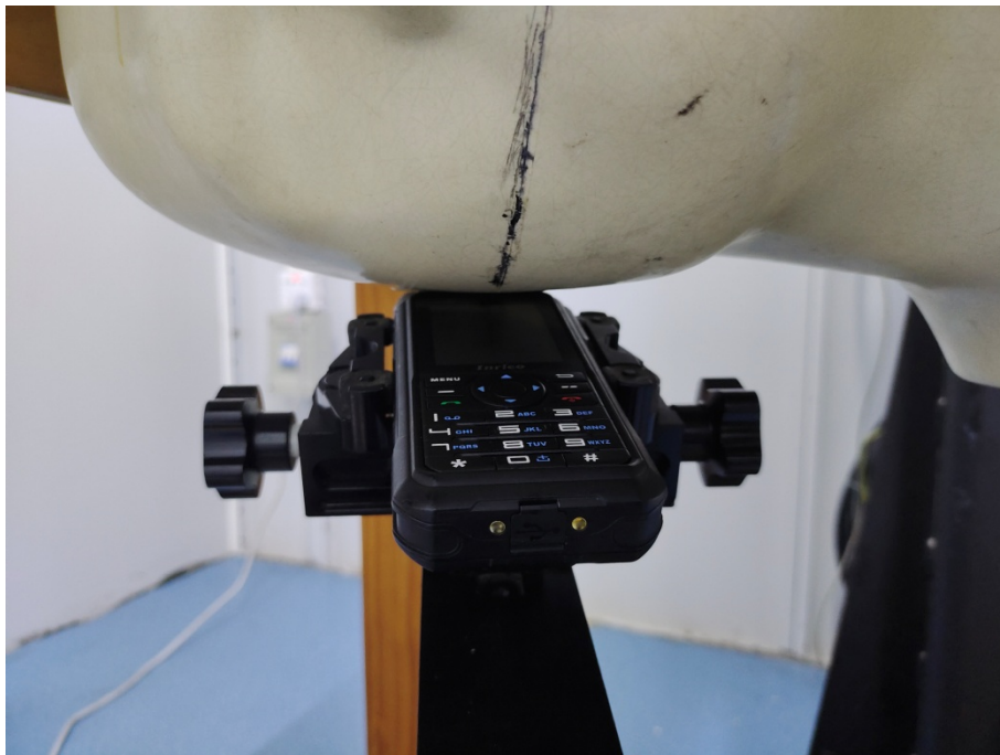
Head Right Tilt Setup Photo (0mm)
