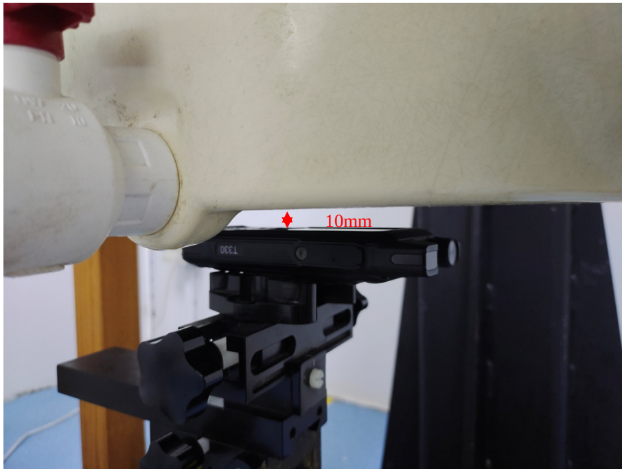
Body(Worn) Back Setup Photo (10mm)
