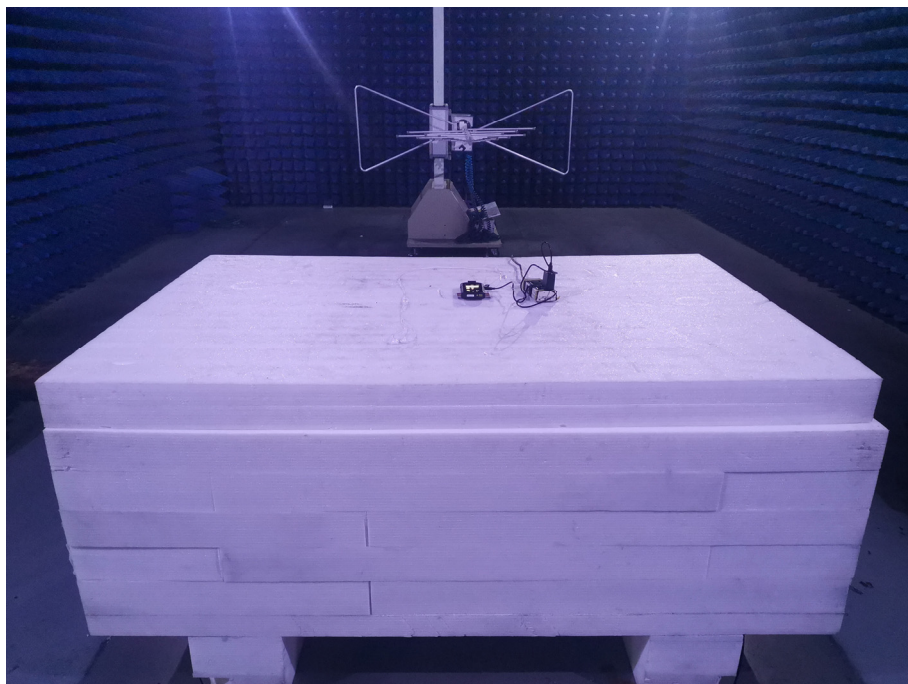
Photo of Radiated Emission Measurement (30MHz-1GHz)
