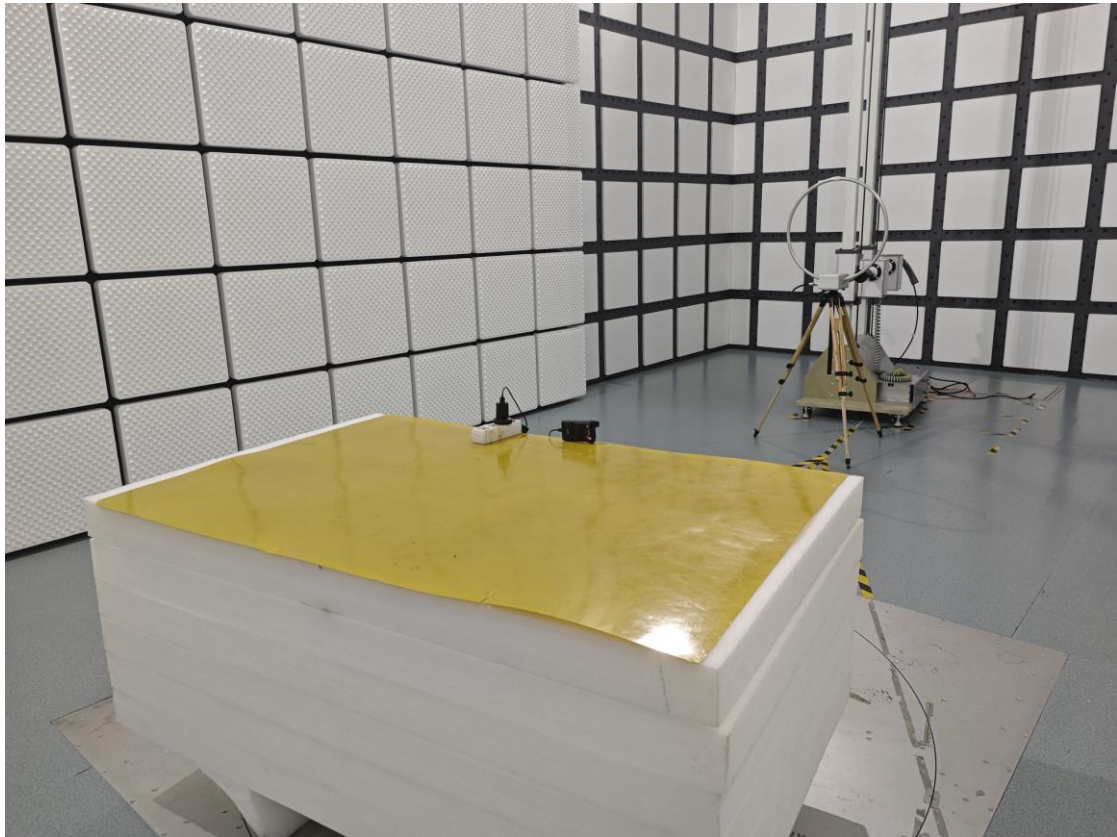
Radiated Spurious Emissions Test View (30MHz-1GHz)-Without Card
