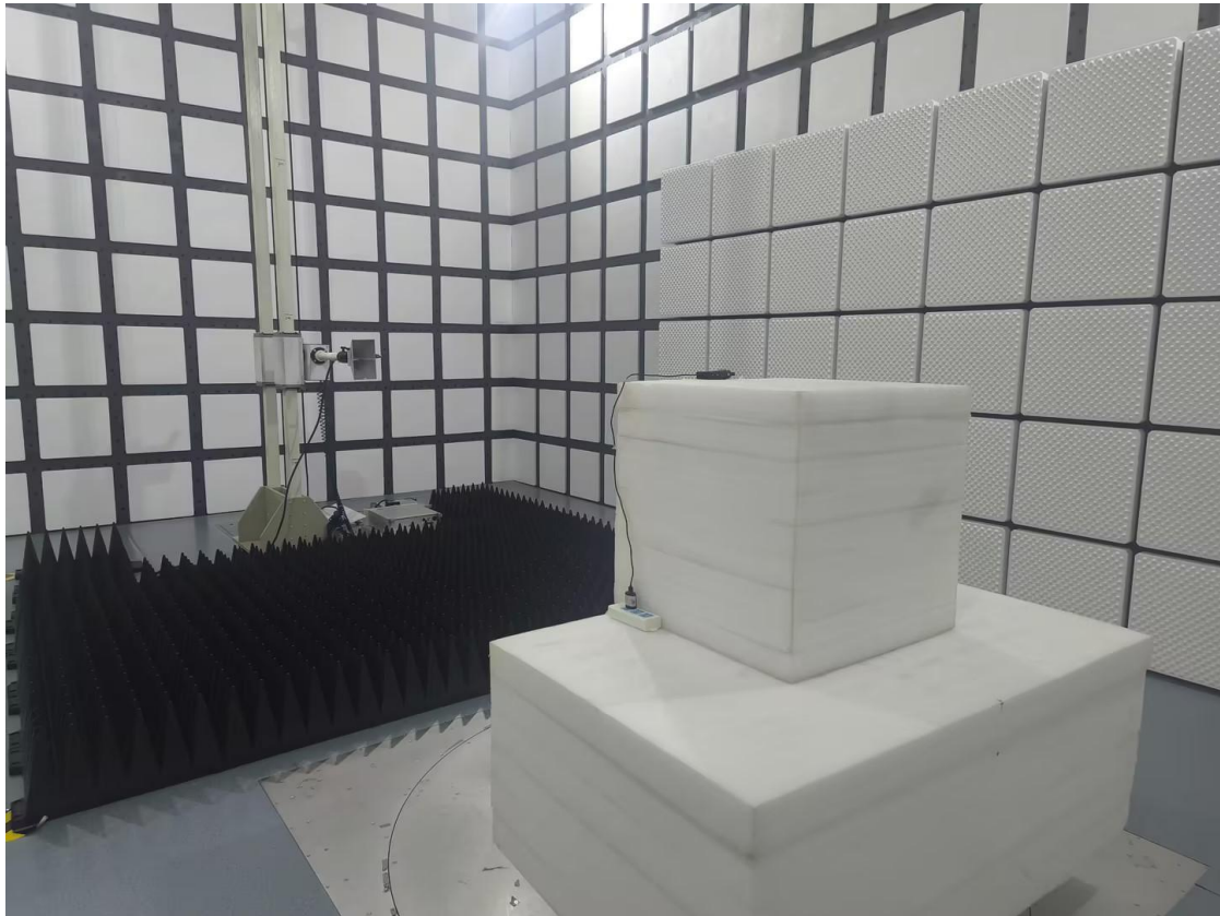
Radiated Spurious Emissions Test View (Above 18GHz)-Adapter
