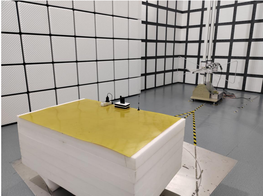
Radiated Spurious Emissions Test View (Above 1GHz)
