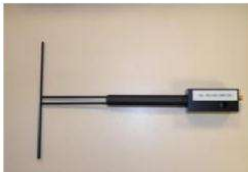
Figure 1 – Satimo COMOSAR Validation Dipole
