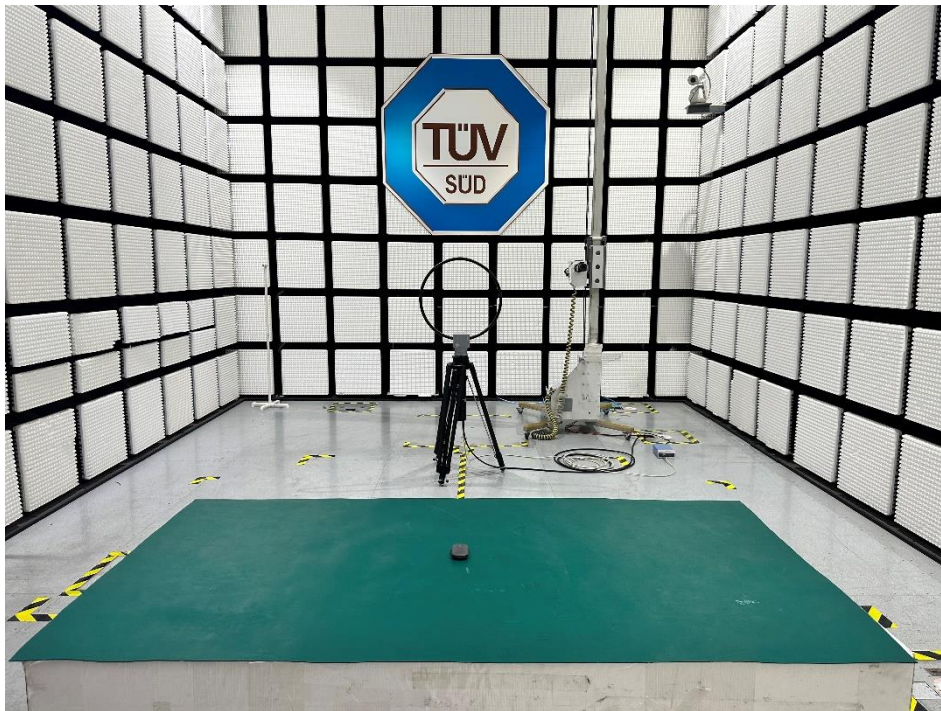
Radiated Emission Setup 9kHz ~ 30MHz
