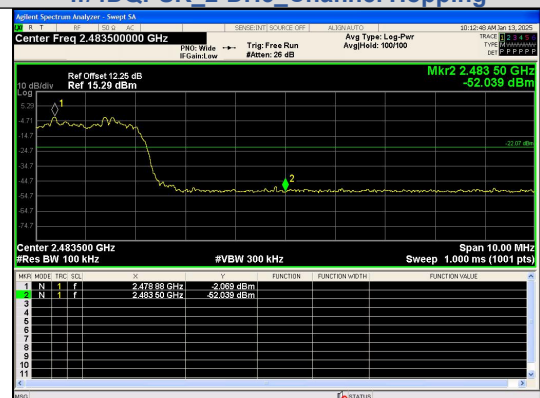
Out Of Band Emission(Right) \pi/4 DQPSK_2-DH5_Channel Hopping
