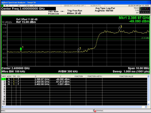
Out Of Band Emission(Left) \pi/4 DQPSK_2-DH5_Channel Hopping
